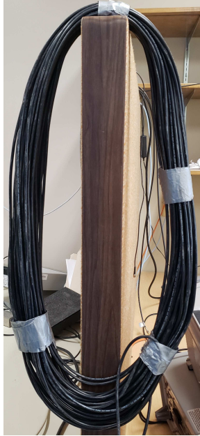
Figure 7.5 Hung Cable for Experiment on Lightly Shaking
