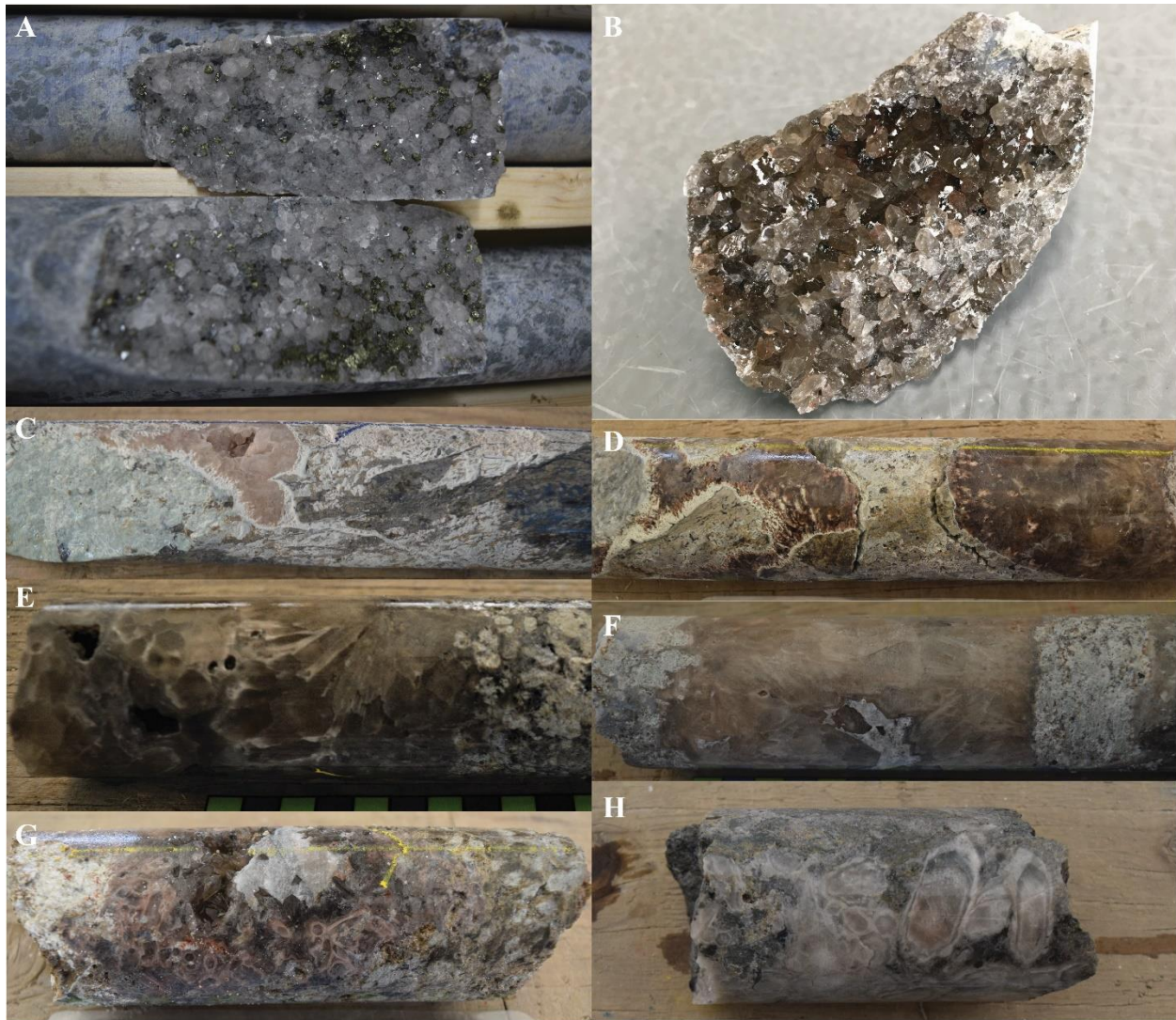
Fig. 5.4. Spectrum of different quartz habits and colors encountered within the Arrow zone as breccia matrices and crosscutting hydrothermal veins or void fill. A) Crosscutting translucent drusy quartz vein with late euhedral pyrite and chalcopyrite mineralization (AR-16-071, 768.0 m). B) Smoky translucent drusy quartz vein proximal to uranium mineralization (AR-18-200c1, 627.1 m). C) Drusy pink quartz within a clay-rich hydrothermal breccia 20 m from A1 shear mineralization, with late robin's egg blue dravite along fractures (AR-16-072c2, 418.3 m). D) Mineralized smoky-pink quartz breccia with late clay-dravite alteration rimming clasts and "eating away" at vein margins (AR-16-085c4, 440.0 m, up to 1,130 cps). E) Smoky brown-black euhedral quartz vein adjacent to A2 shear uranium mineralization (AR-16-080c3, 556.6 m, up to 2,000 cps). F) Smoky brown-pink euhedral quartz vein within the A3 shear zone, adjacent to uranium mineralization (AR-16-086c1, 624.0 m, up to 3,900 cps). G) Vuggy, smoky brown-black drusy quartz void fill with pink-red zoning in crystals proximal to A2 uranium mineralization (AR-16-085c4, 470.0 m, up to 600 cps). H) Spectacular zoning in drusy translucent quartz void fill (AR-16-093c2, 467.4 m).
