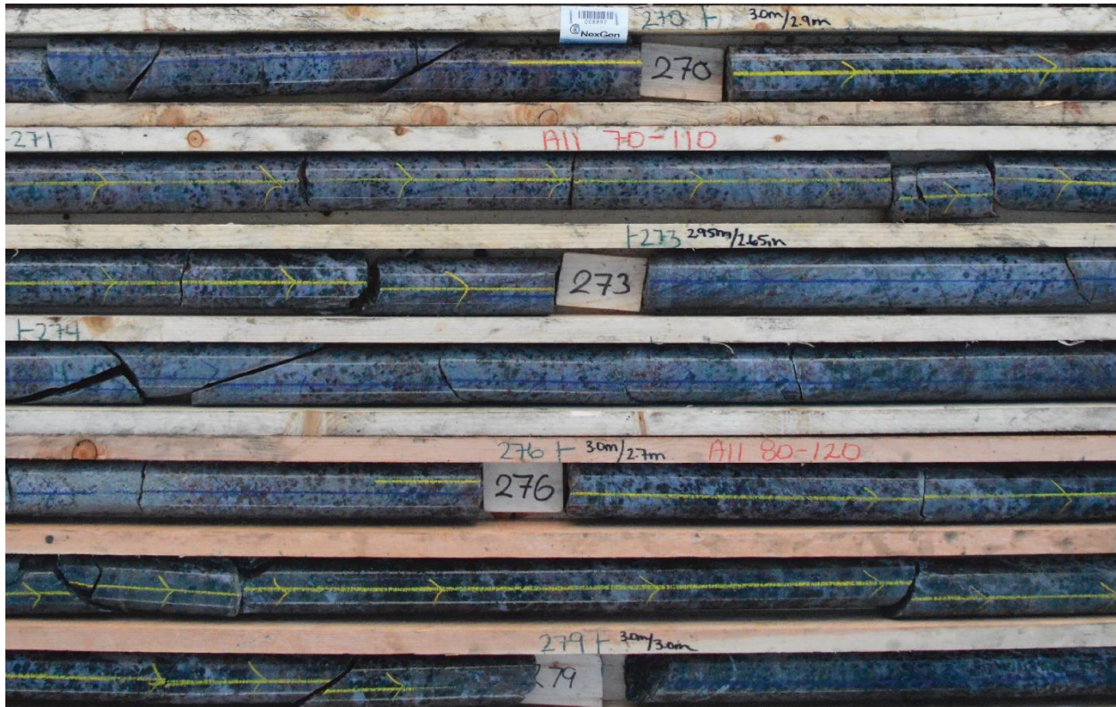
Fig. 3.2. Oriented drill core showing orientation lines (blue and yellow) from four consecutive 3-meter runs in drill hole AR-16-078c2. From 270 to 273 m ( \beta rotation = 350^\circ ), from 273 to 276 m ( \beta rotation = 20^\circ ), and from 276 to 279 m ( \beta rotation = 340^\circ ). Measurements taken from consecutive runs were used for this study.
