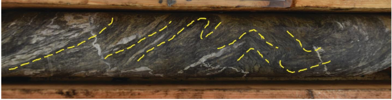
Fig. 4.11. Core photo and fold-trace of a brittle reactivated chloritic-graphitic medium-grade mylonite exhibiting open to isoclinal folding of shear foliations (A1 Shear, AR-16-084c1, 740.6 to 741.0 m, up to 200 cps). Note Brittle reactivation and perpendicular shear fabrics due to F_3 folding and possible F_4 or high strain folding as illustrated in Figure 4.10.
