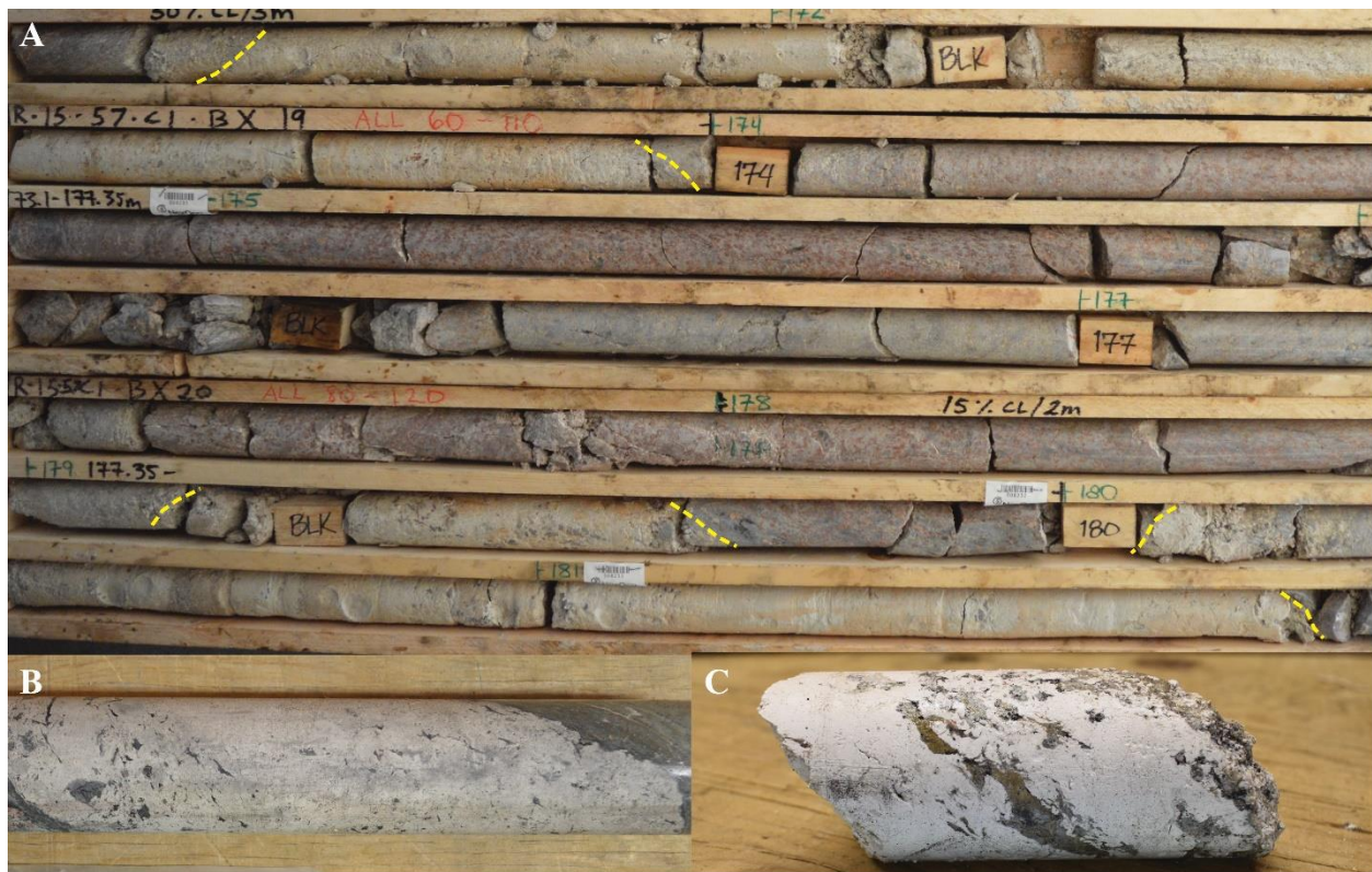
Fig. 4.24. A) Metre-scale cohesive fault gouge zones comprised of >90% kaolinite-illite matrix with negligible clasts of wall rock or quartz. Gouge contacts are annotated by the yellow dashed lines (AR-15-057c1, 171.0 to 181.7 m). B) Mineralized cohesive fault gouge consisting of millimetre- to centimetre-scale clasts of sheared, chloritized and sericitized wall rock within a kaolinite-illite matrix (AR-17-129c1, 764.7 m, up to 5,400 cps). C) Clay-rich cohesive cataclasite hosting weak uranium mineralization. Yellowish-brown and green-blue clasts are pervasively sericitized and/or chloritized wall rock (AR-17-176c1, 506.4 m, up to 600 cps).
