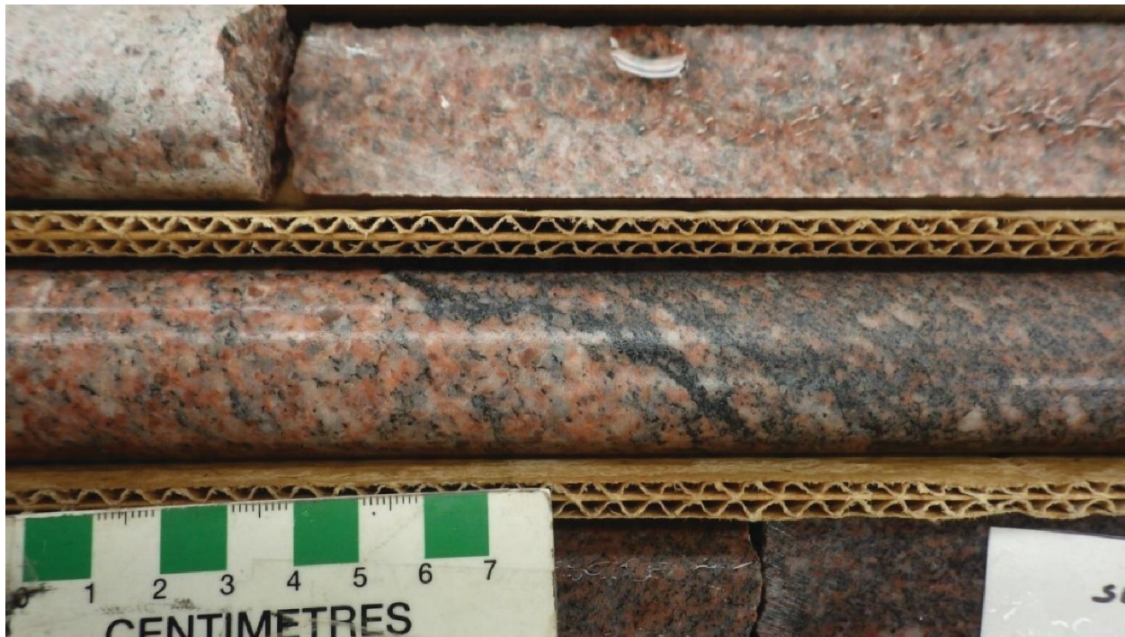
Fig. 2.3. Drill core photo of K-feldspar-rich, gneissic granitoid rock from the Clearwater Domain (From Card et al. 2018).
