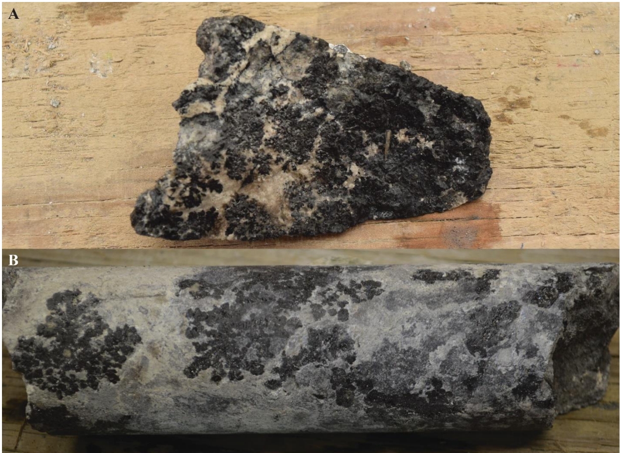
Fig. 6.3. A) Dendritic uraninite (group 1) mineralization along a fracture (AR-16-086c1, 822.2 m, up to 34,000 cps). B) Dendritic patches of uraninite (group 1) mineralization within moderately to strongly clay-altered wall rock (AR-16-076c3, 518.4 m, up to >61,000 cps).
