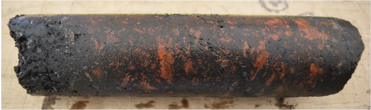
Fig. 6.2. Semi-massive uraninite (group 1) mineralization and associated hematite alteration within the A2 high-grade core (AR-16-093c2, 485.7 to 485.85 m, up to >61,000 cps).
