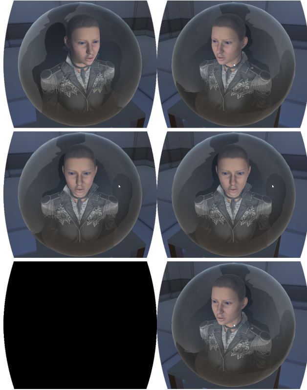
Figure 5.1: An example, with exaggerated stereo disparity, of what the left and right eyes would see in the Stereo (top), NonStereo (middle), and Monocular (bottom) viewing conditions. Note that non-stereo rendering creates a perspective mismatch between the background 3D world and the display.
