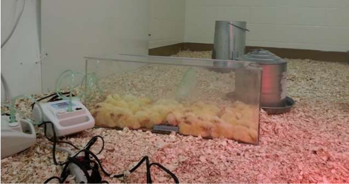
Figure 2.1 Intrapulmonary CpG-ODN administration to a group of 40 neonatal broiler chicks. The acrylic chamber ( 0.036\text{m}^3 ) containing chicks ( n = 40 ) with tubing and mask is attached to a compressor nebulizer set up in the animal room.
