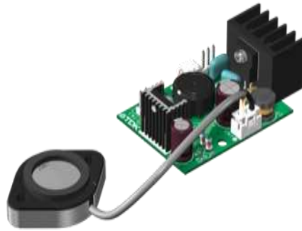
Figure 3.2 An individual ultrasonic type nebulizer Each consisted of a piezoelectric ceramic plate with the ability to generate high frequency ultrasonic waves to convert the CpG-ODN solution into aerosol droplets. An array of these was used.
