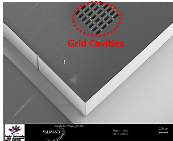
Figure 7.15 a) SEM image of the exposed PMMA demonstrating the side wall and structure quality © 2019 IEEE. Reprinted with permission.
