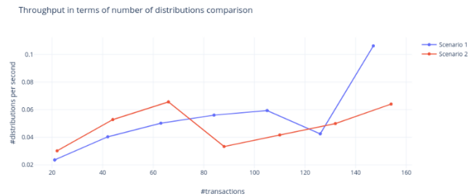
Fig 6.15 Throughput in terms of Distribution per second for both Scenarios using Ethereum Ganache
