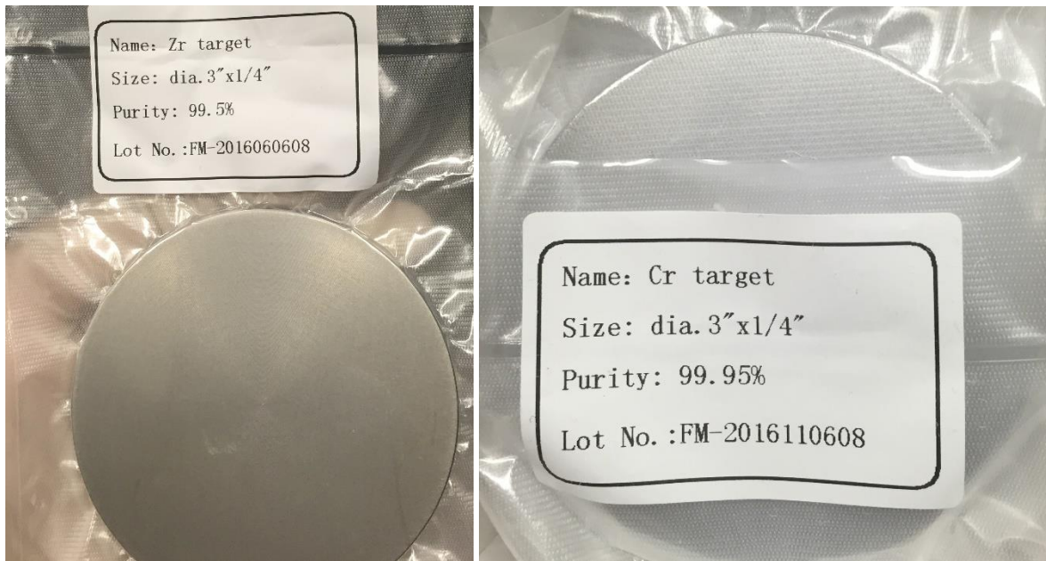
Figure 3-1: Image of Cr and Zr targets with a diameter of 3 inches.
