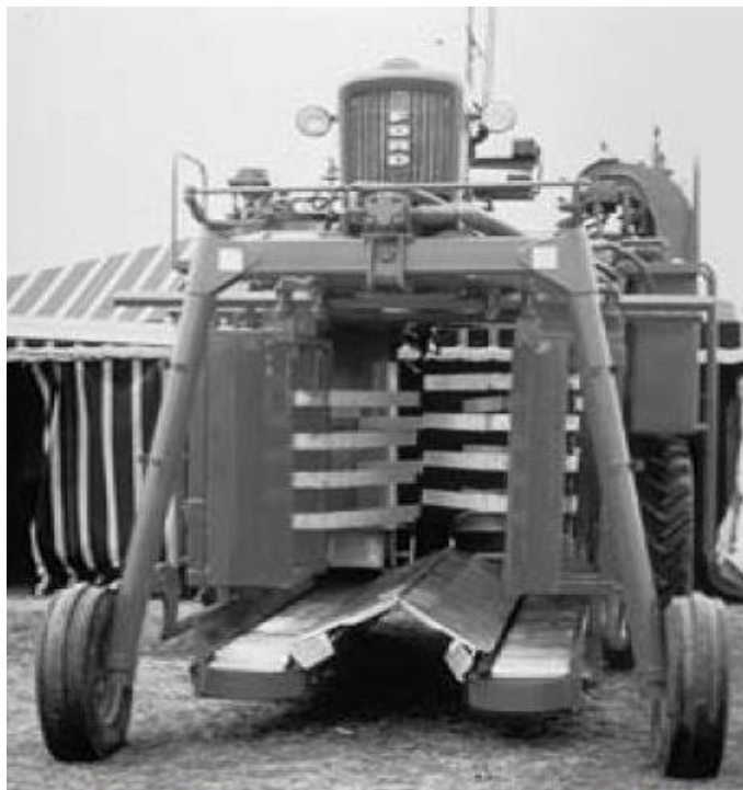
Figure 3.3. Early Chisholm-Ryder Co. grape harvester with flat paddles (Studer, 1969).
