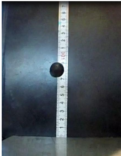
Figure 4.9. Analysis of bounce height for grapes in high-speed video with stainless steel bounce surface.
