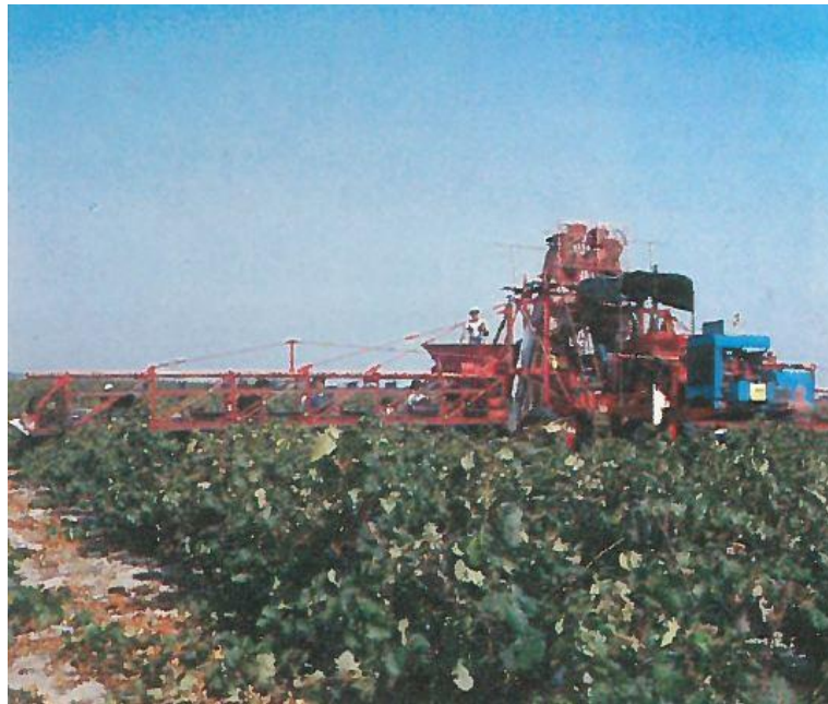
Figure 3.2. Gathering and loading machine for grape harvesting (with permission of Vagny and Agulhon, 1984).
