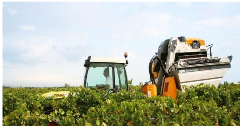
Figure 3.4. Pull-type grape harvester while harvesting in vines (courtesy of Pellenc Group. http://www.pellenc.com/agriculture/ ).
