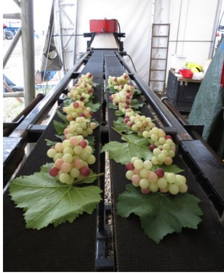
Figure 4.39. Feeding conveyor with leaves and artificial grapes positioned in front of grape harvester test bench.
