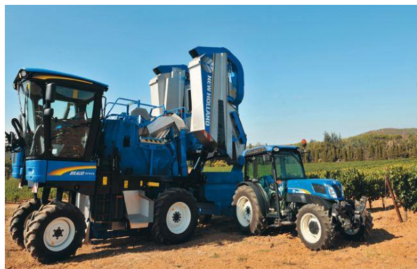
Figure 3.10. Grape harvester emptying storage bins (courtesy of CNH Industrial. http://agriculture1.newholland.com/eu/fr-fr ).
