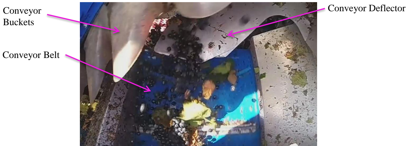
Figure 4.42. Material being propelled in airstream by main conveyor equipped with deflector.
