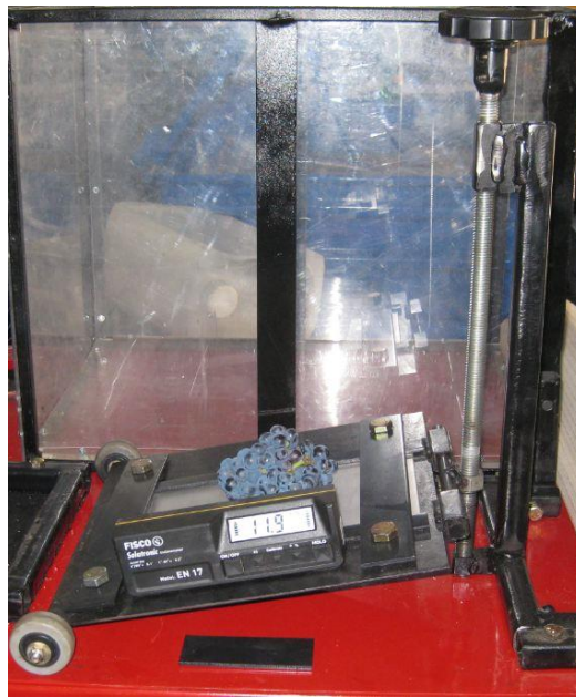
Figure 4.6. Grape bunch and stainless steel surface on inclined plane with digital inclinometer.
