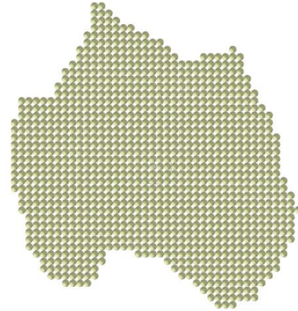
Figure 4.28. Particles placed in uniform grid pattern using coordinates in EDEM ® .
