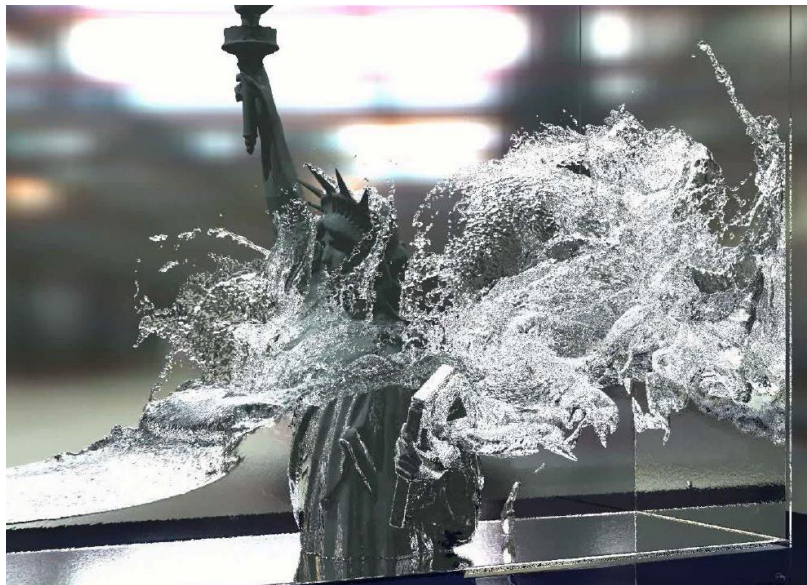
Figure 3.23. DEM simulation of a rogue wave colliding with a statue- 72 million particles with 80 GPUs (Aoki, 2014).
