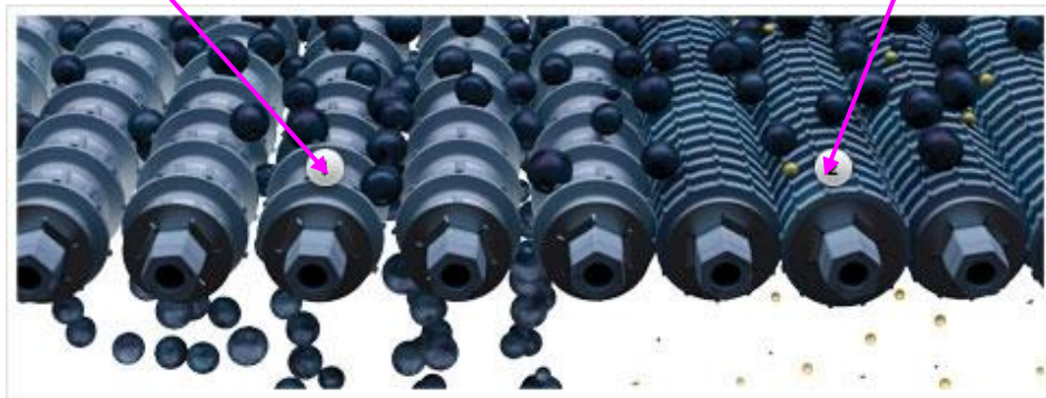
Figure 3.12. Sorting table with sorting rollers (courtesy of Pellenc Group. http://www.pellenc.com/agriculture/ ).
