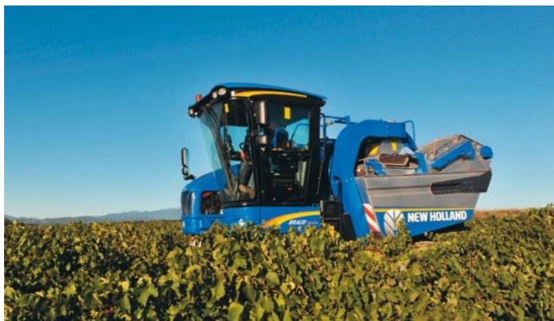
Figure 3.5. Self-propelled grape harvester while harvesting in vines (courtesy of CNH Industrial. http://agriculture1.newholland.com/eu/fr-fr ).
