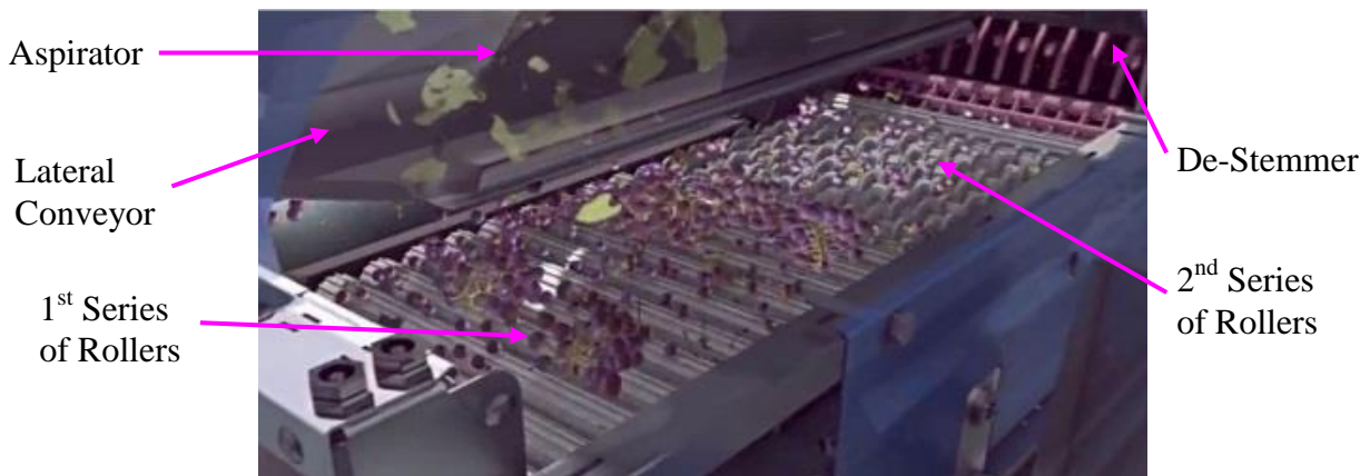
Figure 3.20. Pre-sorter cleaning system with two additional of rollers leading into the de-stemmer (courtesy of CNH Industrial. http://agriculture1.newholland.com/eu/fr-fr ).
