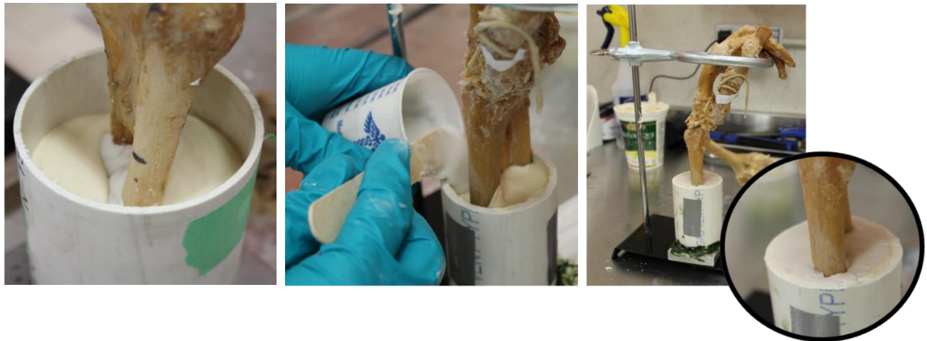
Figure 4-2. Potting specimens with Denstone and securing pot with a layer of polymethylmethacrylate (PMMA). Note, images show a potted embalmed specimen; however, I used fresh-frozen specimens that had soft tissue intact.
