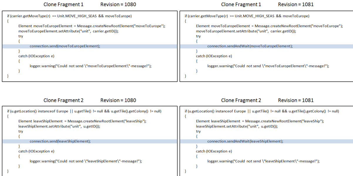
Figure 5.1: Similarity Preserving Co-change (SPCO) example. This figure demonstrates an example of SPCO for two Type 3 clone fragments (Clone Fragment 1, and Clone Fragment 2) in the commit operation applied on revision 1080. We take this example from our subject system Freecol. The snapshots of each clone fragment in the two revisions 1080 and 1081 are shown in the figure, and the changes are highlighted. We can easily understand that in case of each clone fragment, a method named ‘send’ was replaced by a method named ‘sendAndWait’. We see that the clone fragments were changed in the same way. The comment from the programmer regarding this change says that Fixed a potential synchronization bug. “endAndWait” should be used instead of “send” in order to ensure that the server has completed handling the request before we make any modifications to the model. This is a necessary because the server and the AI share the same model. From the changes to the clone fragments and programmer comments we realize that this SPCO is an example of fixing a replicated bug.
