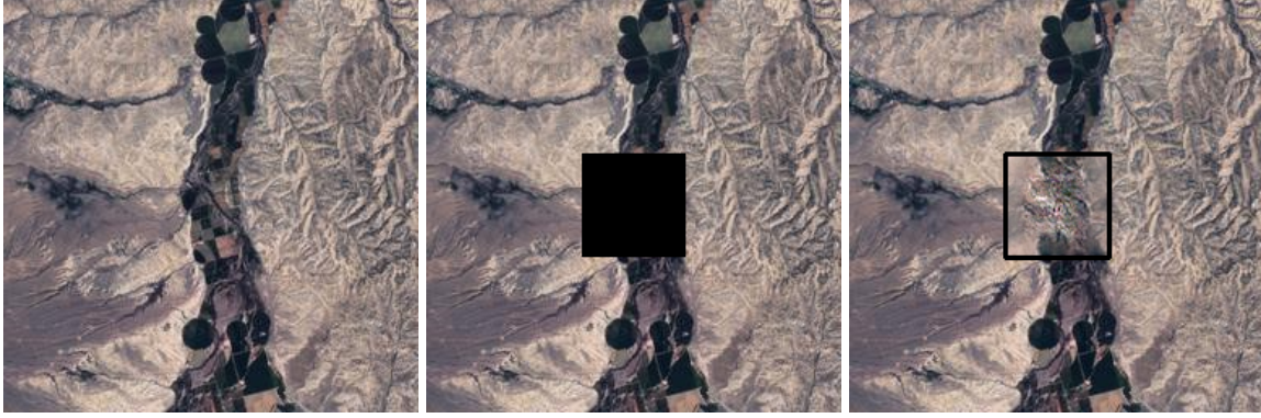
Figure 2.3: (left) Original Image. (middle) The black region shows missing pixels. (right) Image produced by an inpainting algorithm.
