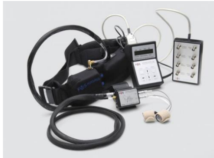
Figure 5-2. The Portapres™ device for measuring continuous BP
