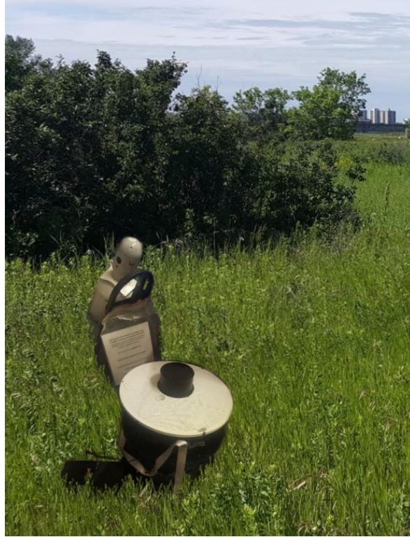
Figure 3.2. Mosquito trap with battery and CO 2 cannister
