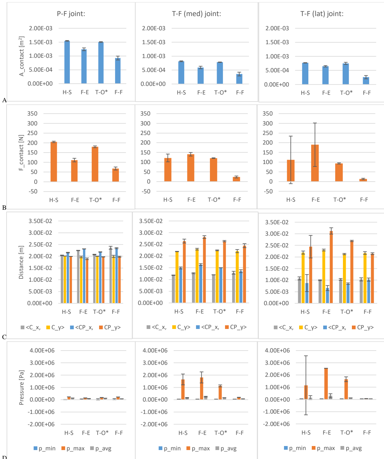
Figure 4-10: Knee loading response repeatability throughout gait (n=3 tests, AVG \pm 2 SD): A. Contact area, B. Contact force magnitudes (compressive), C. Centers of geometry & pressure, and D. Contact pressures magnitudes (compressive). Key gait time points include heel-strike (H-S), full extension (F-E), approximate toe-off (T-O*) and full flexion (F-F). Knee compartments considered are patello-femoral (P-F), and medial and lateral tibio-femoral (T-F,med and T-F,lat).
