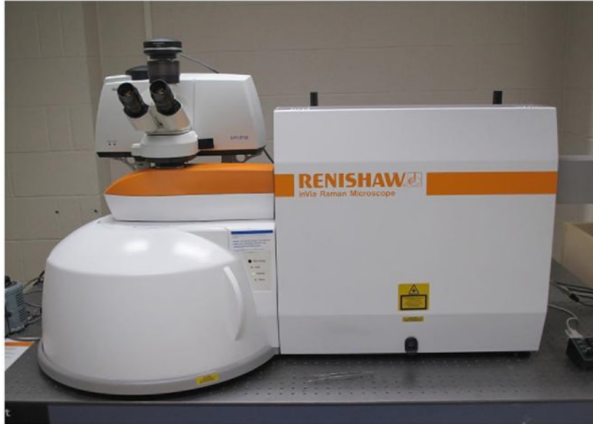
Figure 2.7 Renishaw InVia Reflex Raman Microscope as used in the Saskatchewan Structural Sciences Centre, Vibrational Spectroscopy Laboratory [17].
