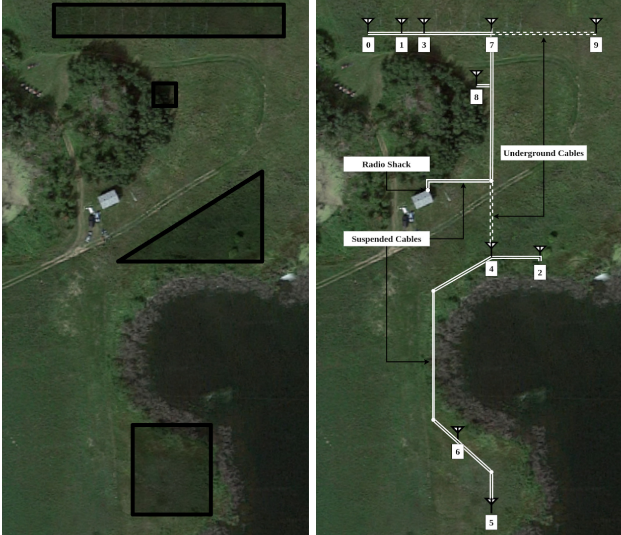
Figure 3.2: (Left) ICEBEAR Receiver site North East of Saskatoon showing areas where antennas are not obstructed by trees, water, buildings, or other experiments. (Right) The final layout of the receiver antenna array, annotated to show antenna numbers, buried cables, and suspended cables. Image acquired from Google Maps, 2020.
