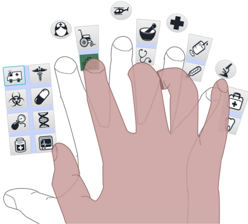
Figure 18: Single-handed selection process (the menu is shown when the hand touches the surface; then user lifts hand and selects item with forefinger).
