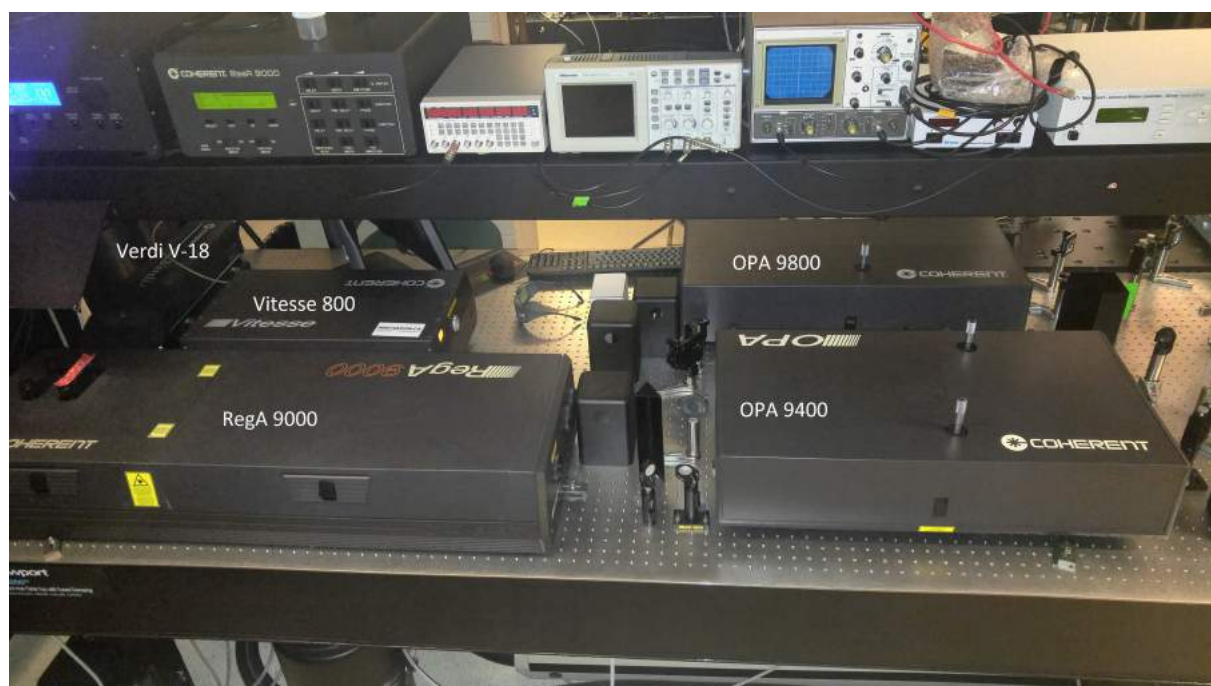
Figure 4.1: Photo of the SSSC SEE laser facility at the University of Saskatchewan. The Verdi, Vitesse, RegA, and OPA units are shown and labelled.
