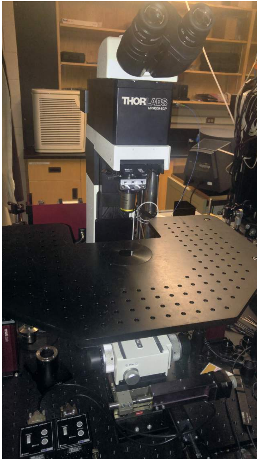
Figure 4.3: Photo of the ThorLabs MPM200-SGP microscope and stage. The 50x objective lens is also visible in the picture.
