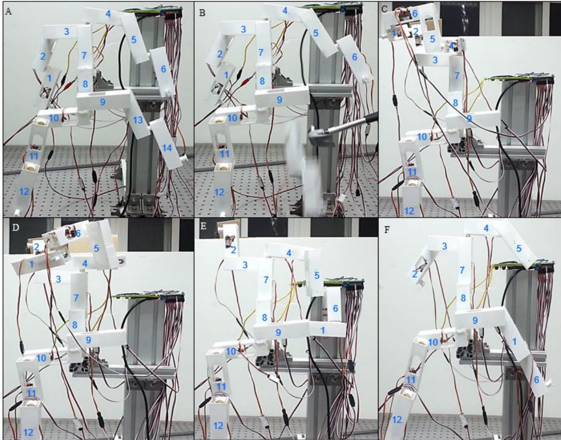
Figure 6.9. Snapshots for a self-reconfiguration trial with the same reconfiguration process as in Figure 6.7: Module 6 picks up Module 1 and assembles it with Module 9.
