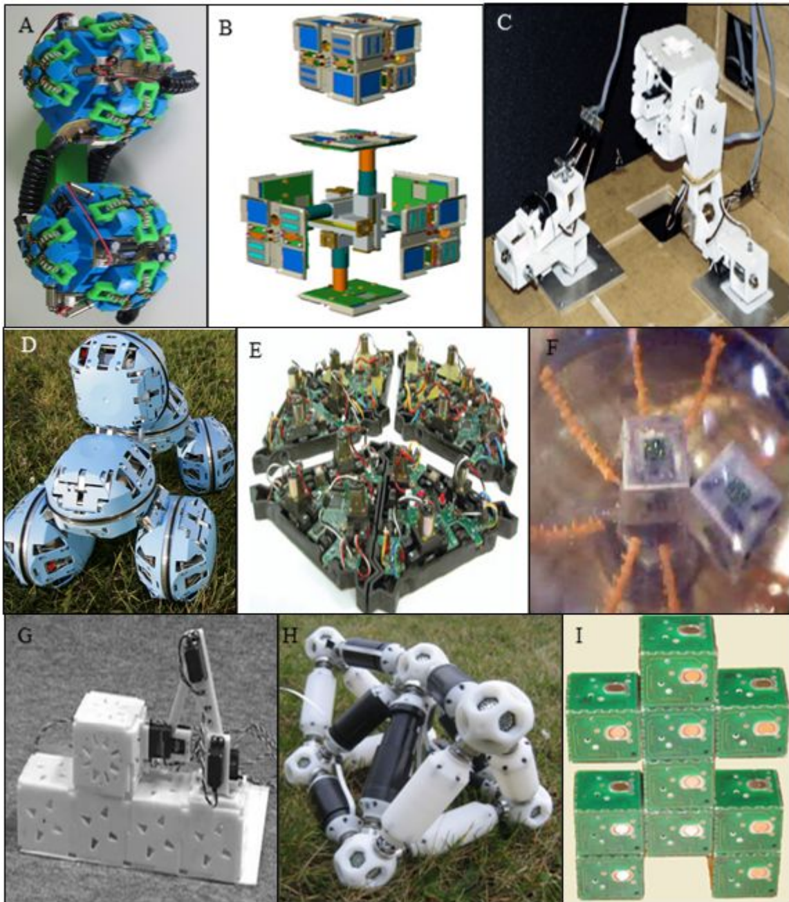
Figure 2.3. Examples of the lattice-type self-reconfigurable modular robots. (A) Molecule [Kotay et al. 1998]. (B) Telecubes [Suh et al. 2002]. (C) ICubes [Unsal and Khosla 2001]. (D) ATRON [Christensen 2006]. (E) The Programmable Parts [Bishop et al. 2005]. (F) Stochastic-3D [Lipson et al. 2005]. (G) A bipartite robot [Terada and Murata 2008]. (H) Odin [Garcia 2008]. (I) Miche [Gilpin et al. 2008].
