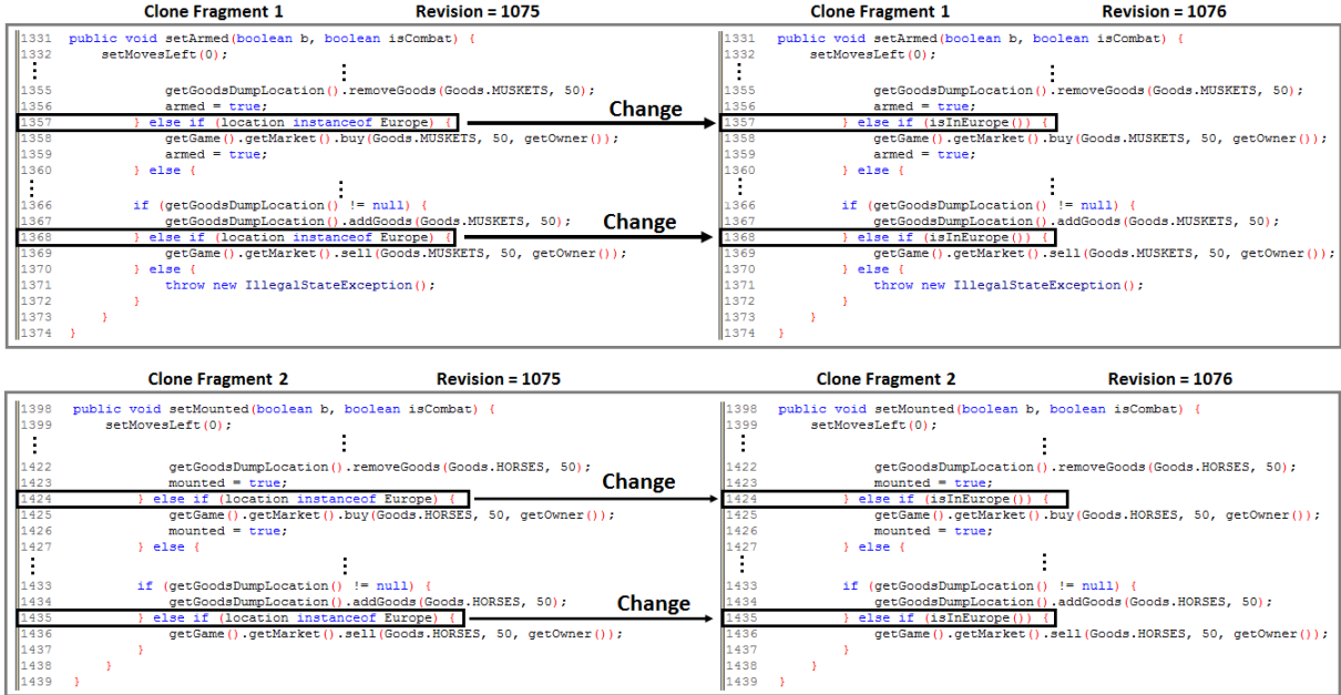
Figure 6.4: An example of a similarity preserving co-change of two Type 3 clone fragments (i.e., Clone Fragment 1, and Clone Fragment 2) of Freecol in a bug-fix commit operation applied to revision 1075. Each of these two clone fragments is a method clone (i.e., the whole method is a clone fragment). The figure shows that they were changed consistently in the bug-fix commit and were again considered as Type 3 clones of each other in revision 1076.
