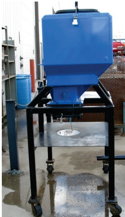
Figure A-3: Product holding tank and metering box before conversion to stepper motor drive.
