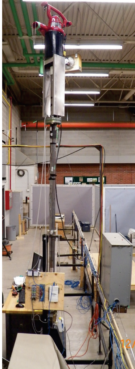
Figure A-2: Powered gas-extraction system as seen from the top of the product tank.
