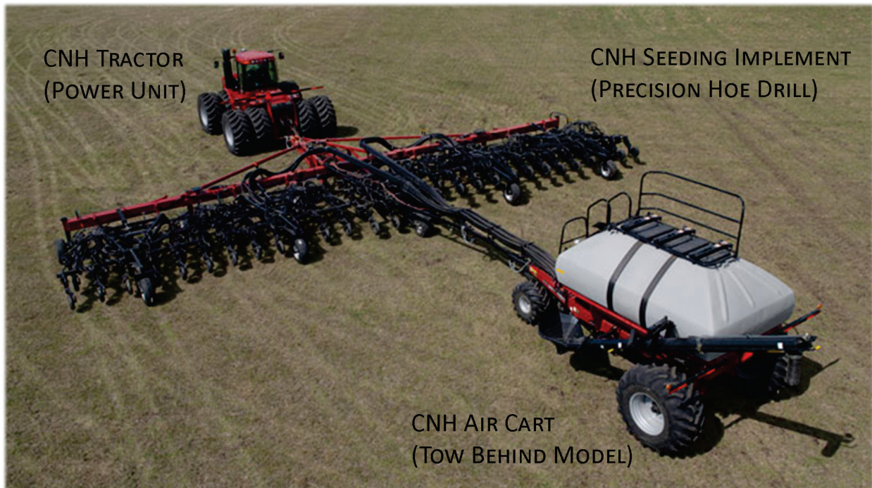
Figure 1.1: CNH seeding implement with tractor, Precision Hoe Drill, and air-cart. Adapted from Case IH 2012 with permission. (Case IH 2012)
