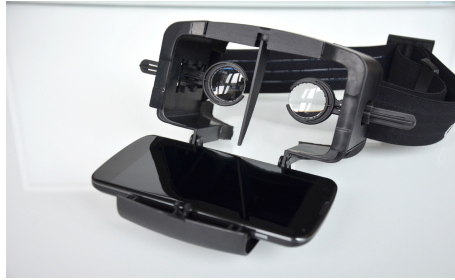
Figure 4.1: Durovis Dive HMD system
