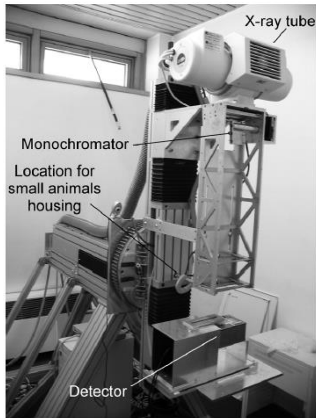
Figure 4.4: A picture of a multi-energy x-ray system for small animals. Source: Ref. [139].
