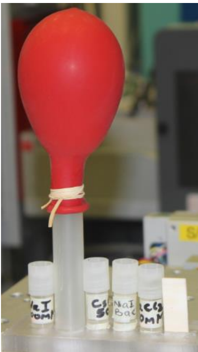
Figure 5.8: Phantom imaged constituting of six materials: starting from left to right: NaI, Xe, CsCl, a mixture of BaCl 2 and NaI, BaCl 2 , and ‘physics bone’-simulated bone (hydroxyapatite in a plastic matrix). Source: Ref. [178].
