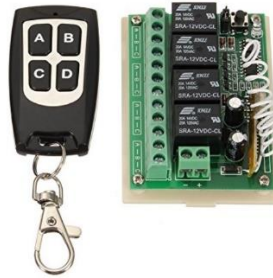
Figure 4-11. A wireless remote control system
