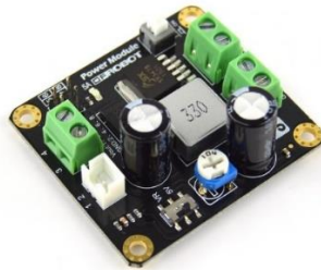
Figure 4-12. A DC-DC Step Down Converter
