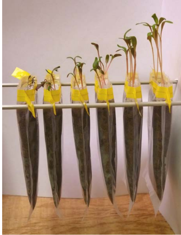
Fig. 2. A 7-d sugar beet biosassay performed in WhirlPak™ bags in the pyroxasulfone concentration range from 0 to 184 ppb.
