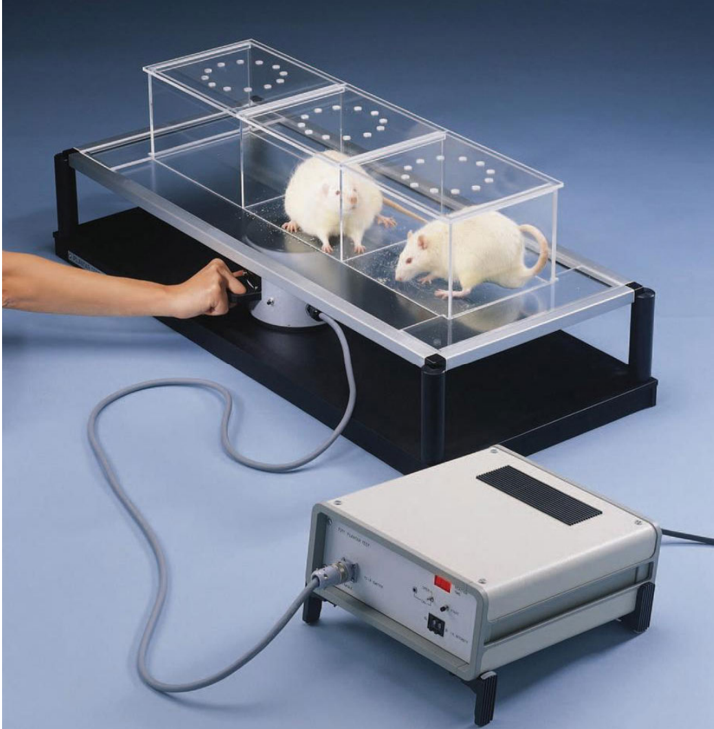
Figure 3.3.1 Thermal hyperalgesia testing apparatus. The Hargreaves testing apparatus consisted of three plexiglass chambers (22 cm long by 17 cm wide by 14 cm high each) on a raised plexiglass floor. An infrared heat source was placed in the center of the hind limb footpad producing heat with a timer running simultaneously. The withdrawal time of each hind limb from the heat source was recorded five times per testing session with a 5 minute rest period between each hind limb recording.
