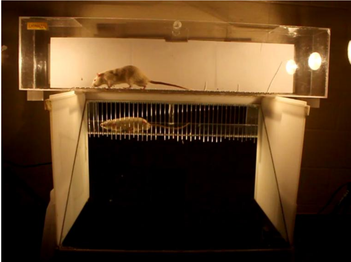
Figure 3.3.3 Ladder crossing testing apparatus. The ladder crossing testing apparatus was custom-made out of clear plexiglass and measured 80 cm long with 20 cm opaque platform at each end. Two millimeters metal pegs are evenly spaced by 1 cm along the track. It sits above an angled mirror so that video recordings can show the animal's positioning as well as their hind limb and toe placements on/between the pegs. Ten ladder crossings were recorded per testing session.
