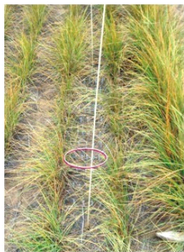
Fig. 1. Experimental set up in one plot. One row of bait-lamina strips (as shown in the circle) is an experimental unit. Each of six rows contains one different bait flavour. Strips in other rows were used to determine the most appropriate removal time.
