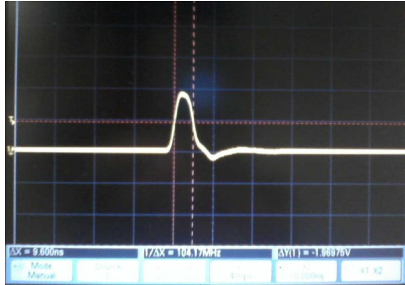
Figure 4.7 Photograph of the SET pulse at the output of the dual-well comparator. The grid for x-axis is 1ns, for y-axis is 0.5V.
