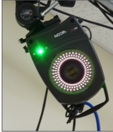
Figure 2.12: A motion capture camera used by an optical motion capture system.
