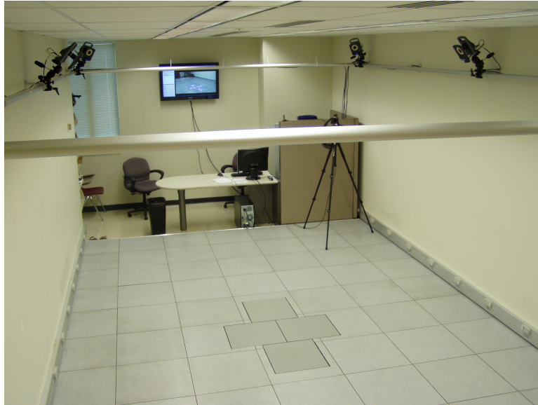
Figure 2.11: A motion capture lab. Note the track-mounted motion capture cameras in upper part of the image.(Image used by permission from the Human Balance and Ambulation Research Laboratory at the University of Missouri - Kansas City)
