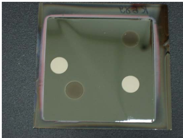
Figure 4.5 A photo of a sample from sample set D with round Al (light) and Pt (dark) contacts on each side. The reflection of light from the ridge dividing the thick and thin sides can be seen.
