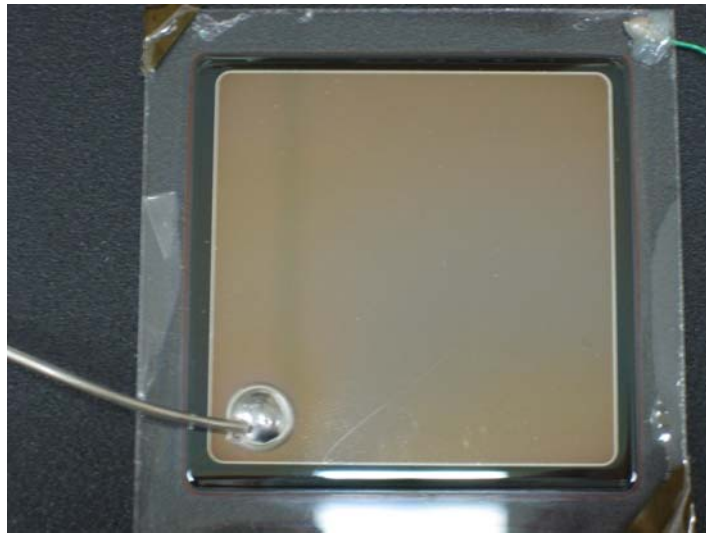
Figure 4.2 A Photo of a sample from sample set A. The entire top surface of the sample is covered by a Cr contact.
