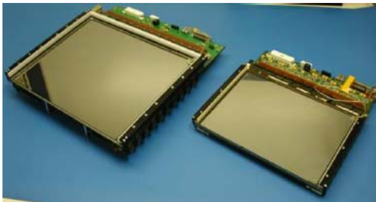
Figure 1.6 a-Se based, direct conversion x-ray image detectors without their protective, light proof cases.
