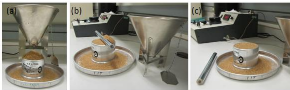
Figure 4.2. Procedure of measuring volume of particles in bulk density measurement
