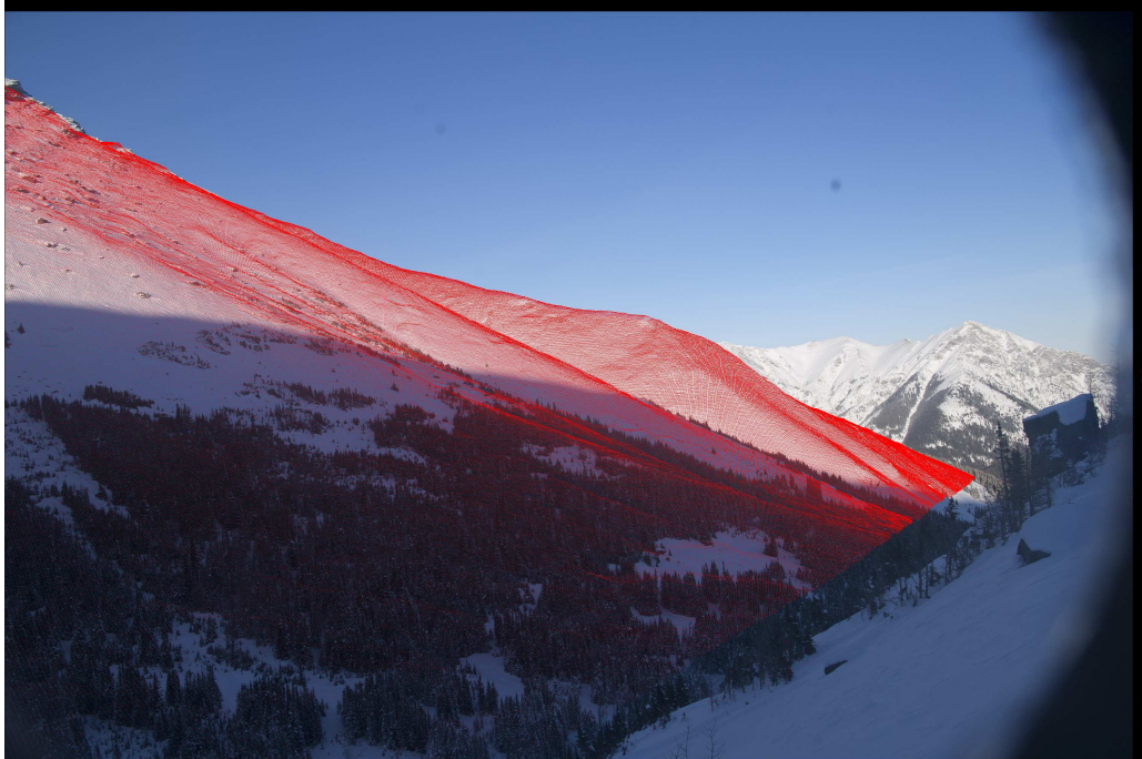
Figure 3.2: Example of the orthorectification perspective transform of the 1\text{ m} \times 1\text{ m} DEM (red points). The perspective transformed DEM is shown on top of the unprocessed timelapse photography take at Fisera Ridge North, Feb. 1st, 2011 at 17:00. The computed viewshed (not shown) causes the sharp edge in the transformed DEM.
