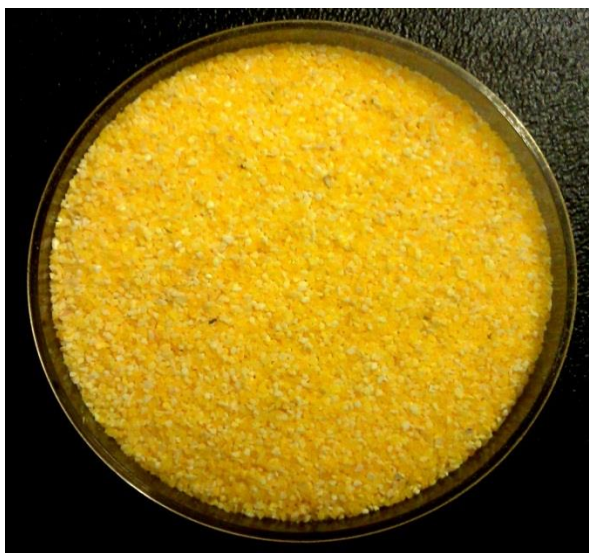
Figure 3.3 Corn meal with particle sizes 0.425-1.18 mm.
