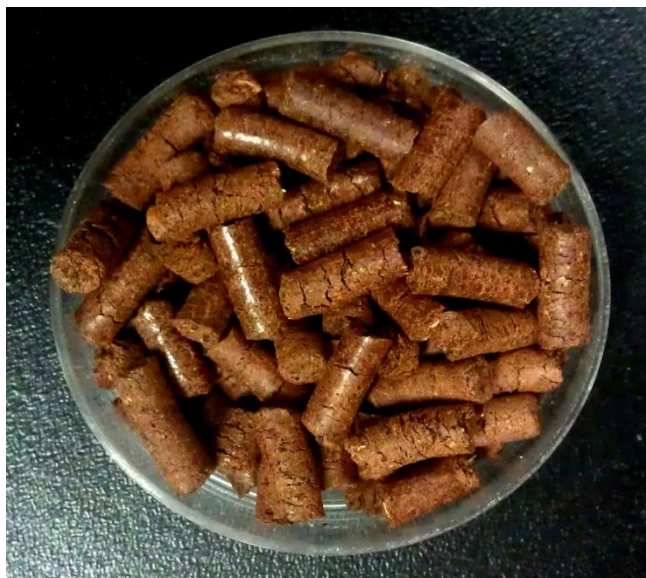
Figure 3.2 Cylindrical pellets with 5 mm in diameter and 10 mm in length.
