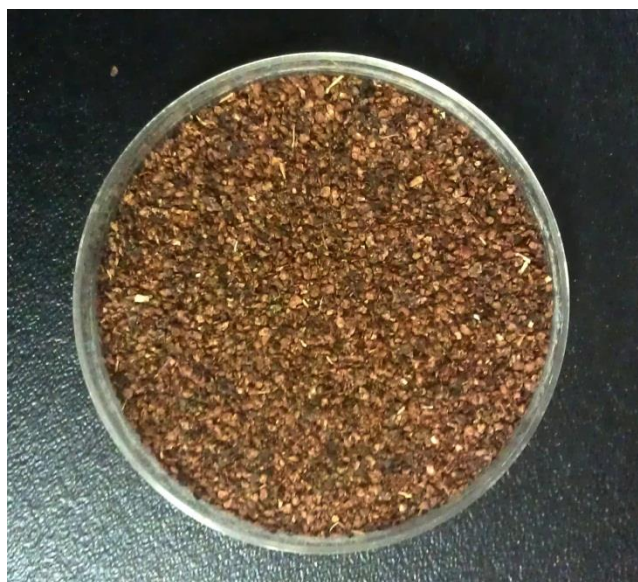
Figure 3.1 Canola meal with particle sizes 0.425-1.18 mm.
