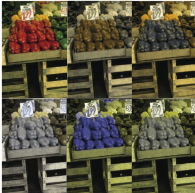
Figure 2.40: Demonstration of Ruminski et al.’s two proposed recolouring algorithms [121]. Top row, left to right: original image, deuteranopic simulated views of Rasche’s recolouring [117] and Kuhn’s recolouring [90]. Bottom row, left to right: deuteranopic simulated views of the original image after Daltonize recolouring [30], Ruminski method one, and Ruminski method two. Images copied from [121].
