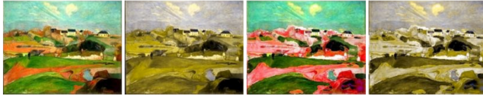
Figure 2.15: Recolouring an image of a painting using Iaccarino et al.’s edge-service tool [67]. From left to right: original image; protanopic or deuteranopic (unspecified) simulated view of original image; recoloured version of original image; protanopic or deuteranopic (unspecified) simulated view of the image after recolouring. Images copied from [67].
