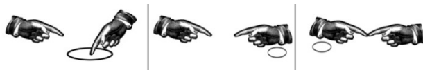
Figure 4.13: An illustration of the ElectroTouch technique, where a handoff occurs only when two hands touch
