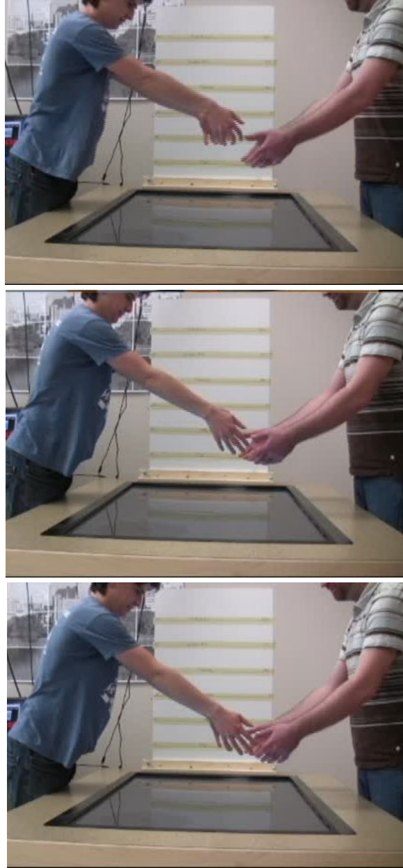
Figure 3.19: Participants transfer a ‘heavy’ box in the Wizard of Oz system. Not only do they maintain the shape of the object but the perceived weight as well. There is a subtle decline in the receiving motion as the receiver (left) compensates for the ‘weight’ of the box.
