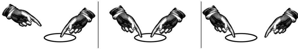
Figure 1.2: An example of a digital object handoff that occurs on the surface. On the left, the giver takes the object and moves it to the transfer zone (middle), where the synchronous exchange takes place and the receiver takes possession (right).
