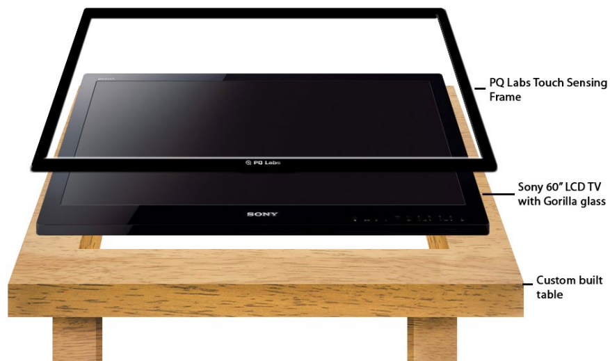
Figure 5.1: The custom built table had the LCD tv inset into the center with a PQ Labs touch frame attached to the top that provided the touch interaction capability.
