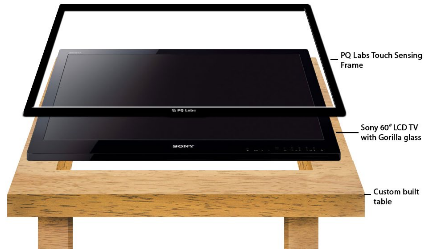
Figure 4.1: A PQ Labs frame is added ovetop a Sony 60" TV with gorilla glass to create a large, mutli-touch display.
