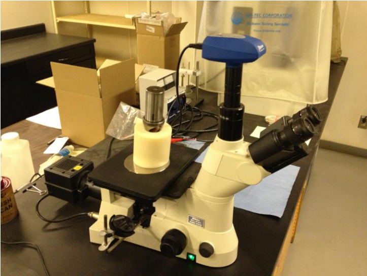
Figure 9: Nikon MA100 Microscope with Drill in Measurement Jig
