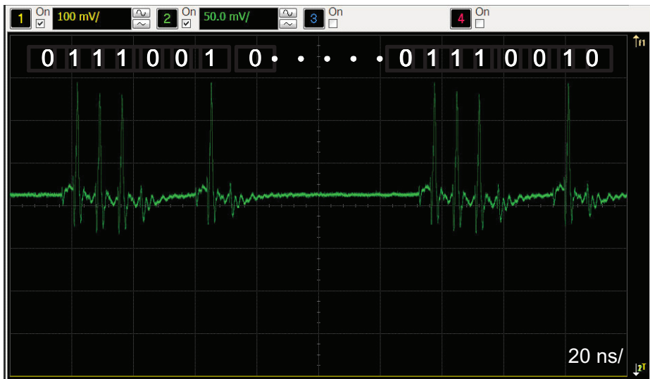
Figure 3.29: Measured transmitter output pulses
