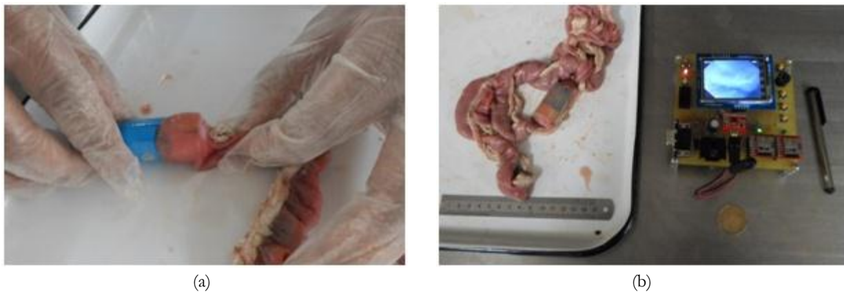
Figure 8.3 (a) Capsule PCBs put in casing and inserted inside pig's small intestine; (b) Experimental setup: capsule inserted in pig's intestine and the data logger is showing real-time inside image of the intestine
