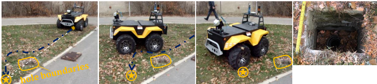
Fig. 5-15: Scenario 3 Snapshots of the robot navigation in point-to-point motion, going in a straight line from the start point (*), left image, to the goal point (⊗) while avoiding a hole. The actual path of the robot is shown in dash-dotted line and the direct path from (*) to the (⊗) is depicted in dash line. Right image shows more detail of the hole.
