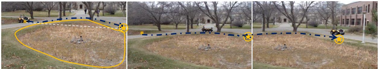
Fig. 5-19: Scenario 5: Snapshots of the robot navigation in point-to-point motion, moving in a straight line from the start point (*), left image, to the goal point (⊛) while avoiding a very big hole. The actual path of the robot is shown in black dash-dotted line and the straight path from (*) to the (⊛) is depicted in white dash line.
