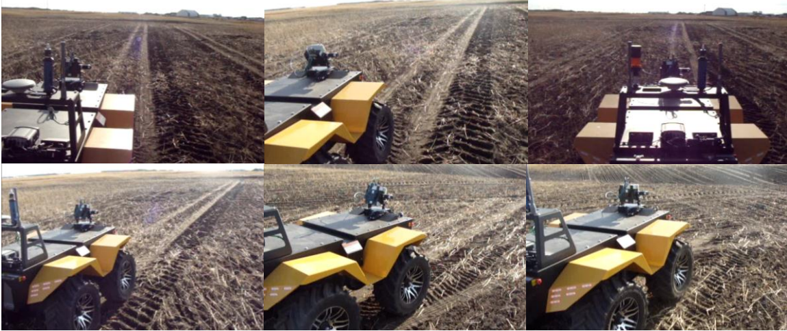
Fig. 5-23: Scenario 7: Snapshots of the robot following a shallow rut in the farm field [19].
