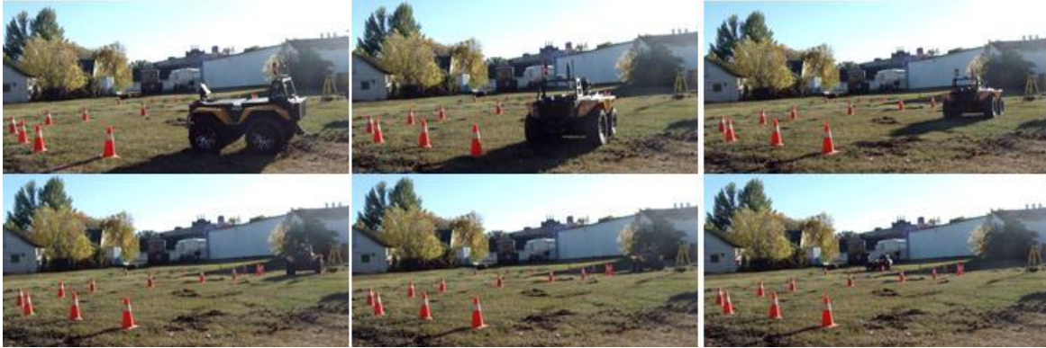
Fig. 4-23: Snapshots of the robot run for experiment in setup8: The robot is traversing from start point to the goal point, using HIM for obstacle avoidance. Top-left: the robot at start point, and bottom-right: the robot at the goal. Image sequence proceeds to the right and down. [22]
