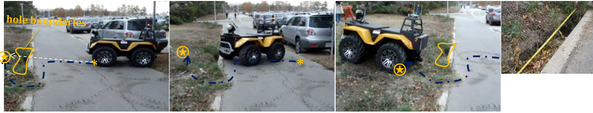
Fig. 5-13: Scenario 2: Snapshots of the robot navigation in point-to-point motion, from the start point (*), left image, to the goal point (⊛) while avoiding a hole. The actual path of the robot is shown in black dash-dotted line and the direct path from (*) to the (⊛) is depicted in white dash line. Right image shows close up view of the hole.
