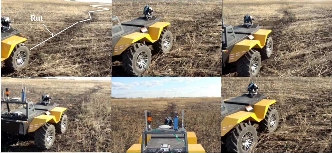
Fig. 5-21: Scenario 6: Snapshots of the robot following a curvy rut in the farm field [19].
