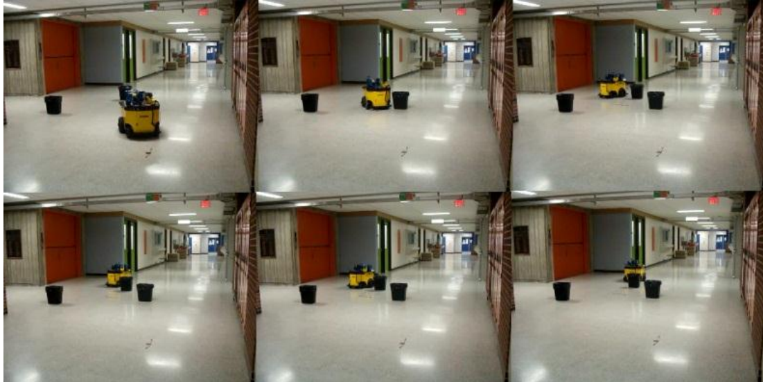
Fig. 3-14: Snapshots of the AGV for experiments. The mobile robot traversing from start point to the goal point, using (a): FLB (b): HIM. Top-left image shows the robot at start point and bottom-right image indicates robot at the goal. Image sequence proceeds to the right and down.
