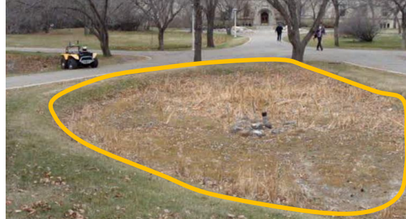
Fig. 5-8: Sample of negative obstacles in off-road terrain
