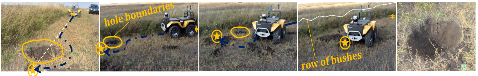
Fig. 5-28: Scenario 9: Snapshots of the robot in proximity-following and hole avoidance test in a farm field [19].
