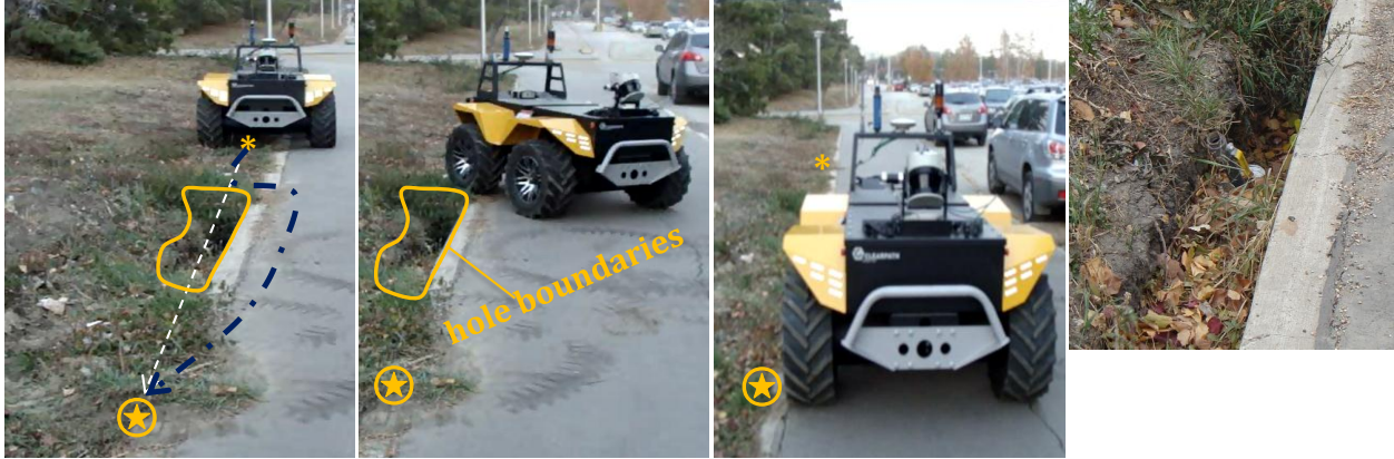
Fig. 5-11: Scenario 1: Snapshots of the robot navigation in point-to-point motion, moving directly from the start point (*), left image, to the goal point (⊕) while avoiding a hole. The actual path of the robot is shown in black dash-dotted line and the direct path from (*) to the (⊕) is depicted in white dash line. Right image shows close up view of the hole.
