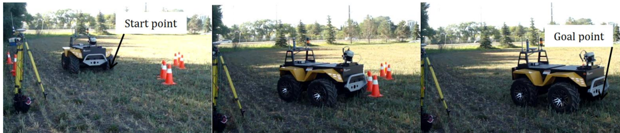
Fig. 4-21: Snapshots of the robot for a typical experiment: The robot is travelling from “start point” to the “goal point”, using HIM for obstacle avoidance. Left: robot at start point, middle: robot at mid-point, right: robot at the goal point in [21]
