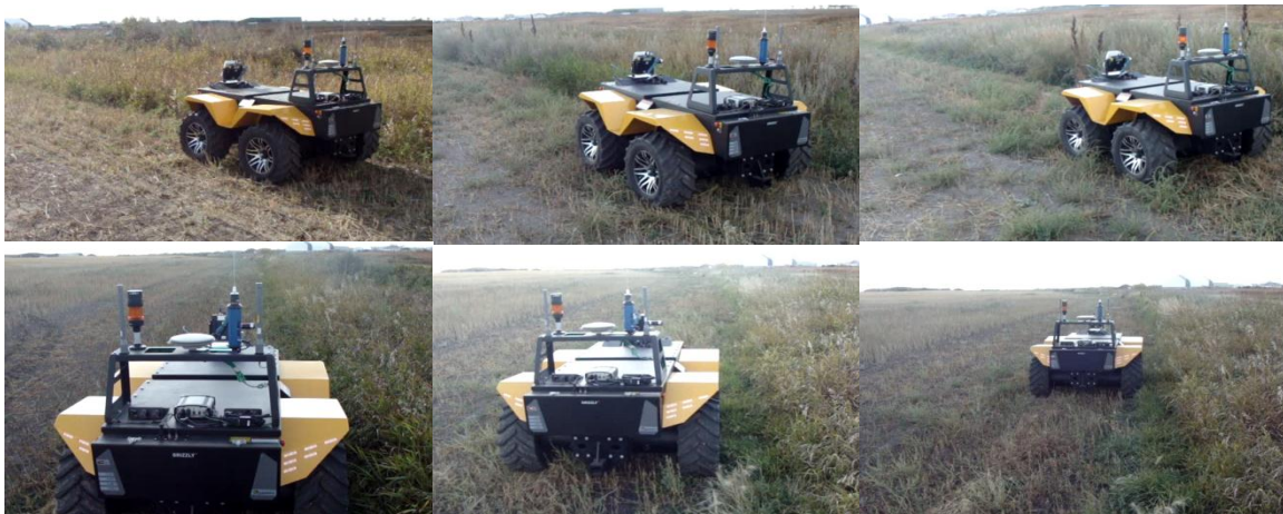
Fig. 5-25: Scenario 8: Snapshots of the robot in a proximity-following test in the farm field [19].
