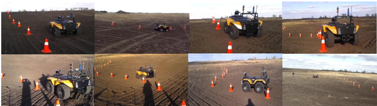
Fig. 4-30: Snapshots of the robot following a path on a hill in [21]. Top-left: the robot at start point, and bottom-right: the robot at the end-point. Image sequence proceeds to the right and down.
