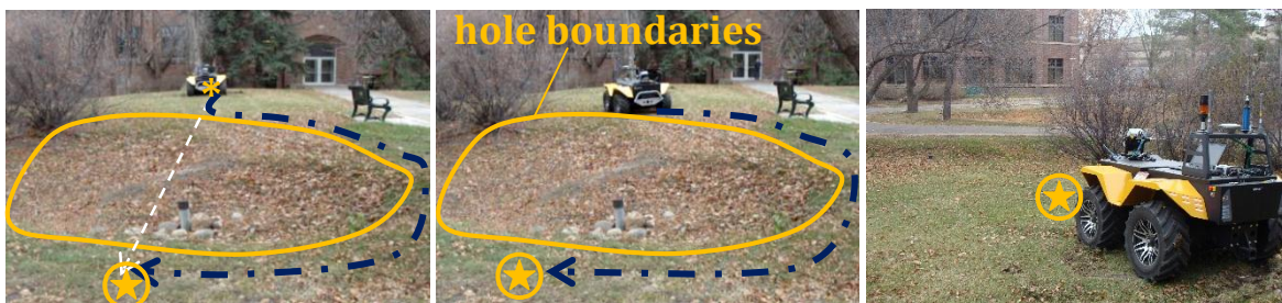
Fig. 5-17: Scenario 4: Snapshots of the robot navigation in point-to-point motion, when moving directly from the start point (*), left image, to the goal point (⊗) while avoiding a very wide hole. The actual path of the robot is shown in black dash-dotted line and the straight path from (*) to the (⊗) is depicted in white dash line.
