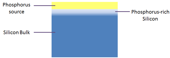
Figure 2.10: Cross-sectional view of phosphorus diffusing into a silicon wafer during PDG. Impurities diffuse from the bulk into the region of phosphorus-rich silicon.
