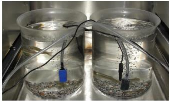
Figure 2-1 – Atlas Suntest XLS+ Solar Simulator set up with 2 L quartz beaker housing fathead minnows placed in a water bath exposed to UVR for 8H a day. Attached airstones ensured constant supply of oxygen and prevented stratification of temperature across the beaker. Digital temperature probes provided a range of the temperature through the entire experiment.
