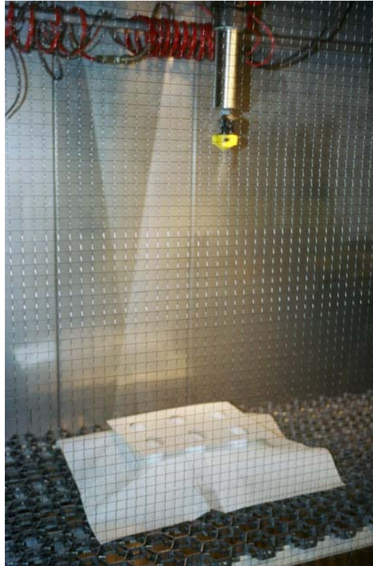
Figure 2-1. Application of commercial 2,4-D formulation onto masked eggs using an agricultural field spray simulator.
