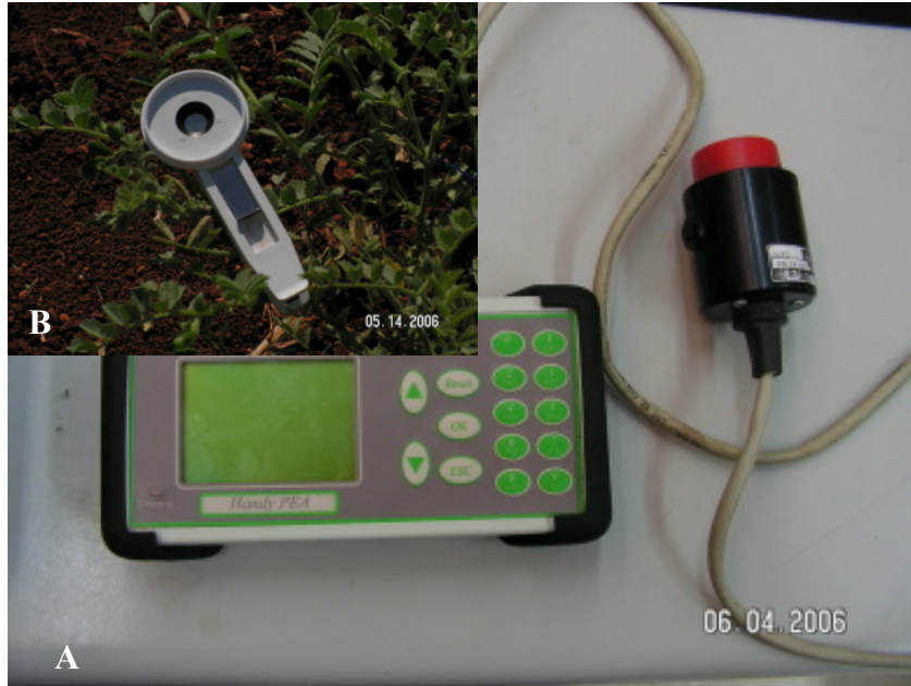
Fig. 5. 1: Chlorophyll fluorescence was measured using (A) Handy PEA (Hansatech Instruments, Norfolk, UK). Clips (B) were fixed on leaves 25 minutes before the measurement for dark adaptation.
