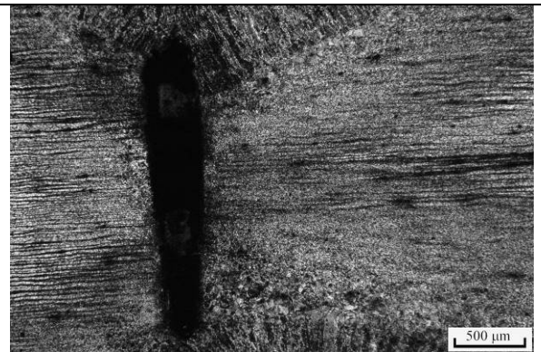
Figure B.14. Interface between the 1 st and 2 nd pass welds for 15.3 mm/s welding speed.
