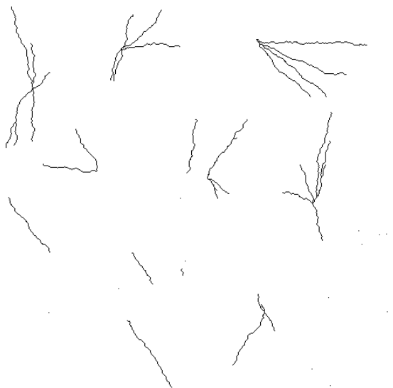
Figure 3.1: This figure depicts a binary image where black pixels correspond to the location of generator nodes. This figure visualizes the input F used for the running example terrain in this chapter.
