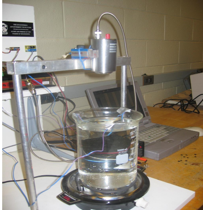
Figure 4.7 Indoor calibration of the thermal infrared sensor
