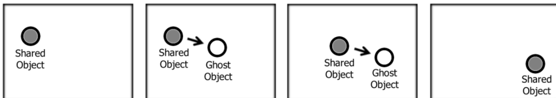
Figure 2.4. The ball is being moved across the screen by the user. In the Echo technique, the ghost object represents immediate feedback while the shared object is updated from the network.
