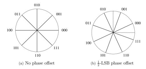
Figure 4.3 Phase wheel comparison between no phase offset and  $\frac{1}{2}$ -LSB phase offset.
