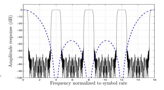
Figure 4.14 Spectral response of 1-to-4 CIC interpolator. Solid line shows the periodic spectrum of the zero packed time series and dashed line shows the frequency response of the CIC filter with rate change factor of 4.
