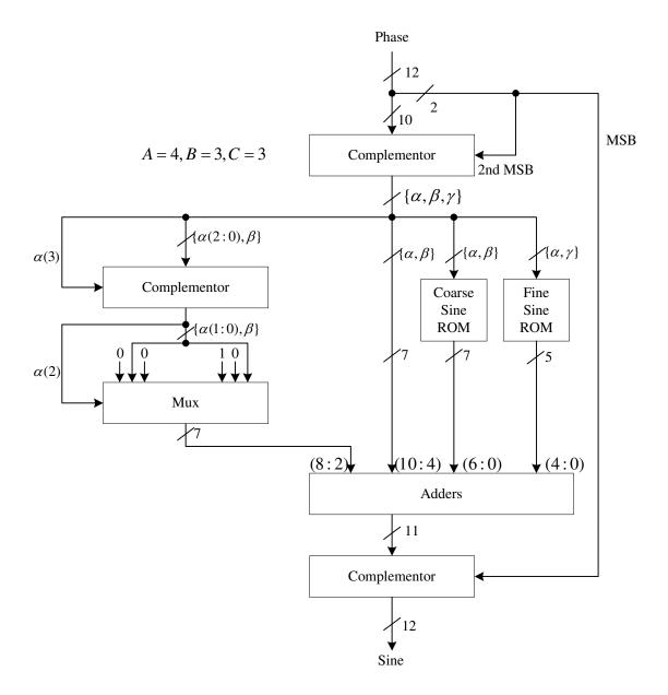
Figure 4.6 Sine phase to amplitude converter using QLA method.
