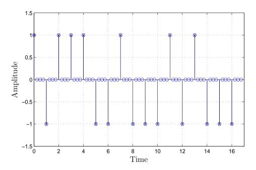
Figure 2.6 An example of 1-to-4 upsampling. "x" shows the input binary data and "o" shows the output after 1-to-4 upsampling.
