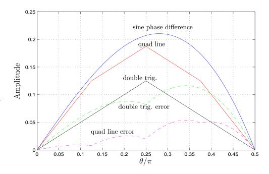
**Figure 4.5** Curves of sine-phase difference, double trigonometric approximation and QLA and the error curves of double trigonometric approximation and QLA.
