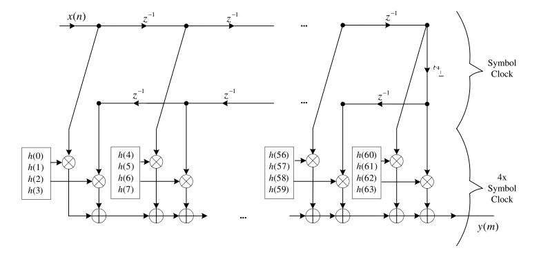
Figure 4.12 Block diagram of the SQRC filter.
