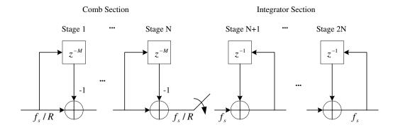
Figure 2.8 Block diagram of the CIC interpolation filter.
