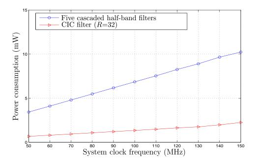
Figure 5.11 Power consumption comparison for two interpolation filters with the interpolation ratio of 32.
