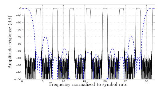
Figure 4.17 Spectral response of three cascaded half-band FIR filters. Solid line shows the periodic spectrum of the zero packed time series and dashed line shows the frequency response of the three cascaded half-band FIR filters.
