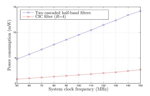
Figure 5.8 Power consumption comparison for two interpolation filters with the interpolation ratio of 4.
