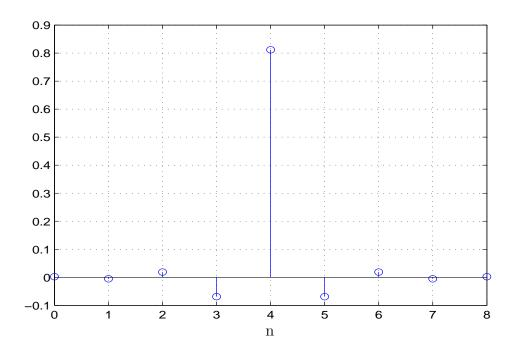
Figure 4.19 Impulse response of the designed inverse sinc filter.
