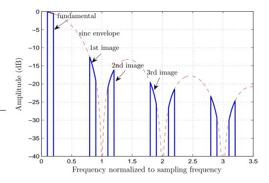
Figure 2.15 Output spectrum of a real world DAC.
