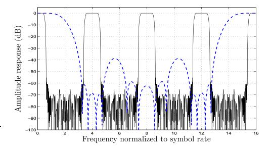
Figure 4.16 Spectral response of two cascaded half-band FIR filters. Solid line shows the periodic spectrum of the zero packed time series and dashed line shows the frequency response of the two cascaded half-band FIR filters.
