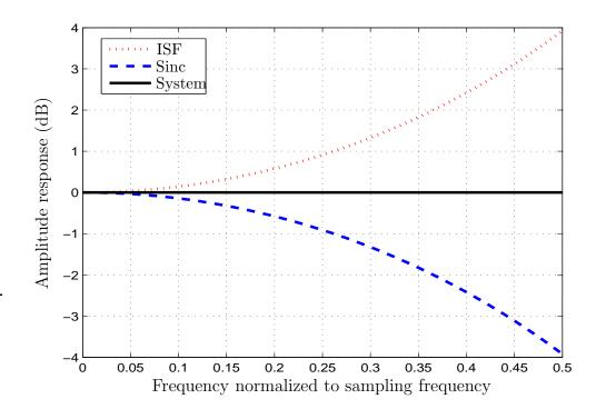
Figure 2.16 Amplitude response of the ideal inverse sinc filter.
