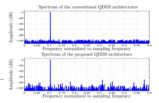
Figure 5.4 Spectrum of the QDDS output  $(f_{out} \approx 0.104 \times f_{refclk})$ .
