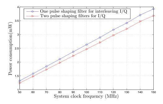
Figure 5.6 Power consumption comparison for 2 different pulse shaping filter implementations (interpolation ratio of interpolation filter=4).
