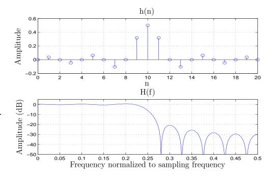
**Figure 2.9** Impulse response and frequency response of a half band FIR filter with the length of 21.
