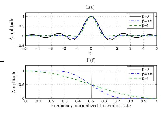
Figure 2.4 Raised cosine pulse and spectrum.
