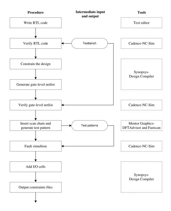
Figure 3.1 Block diagram of the front-end design flow.
