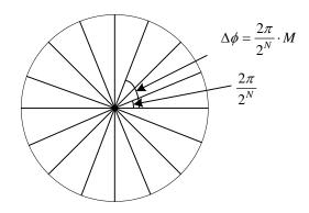
Figure 2.3 Digital phase wheel. As the vector rotates around the wheel, a corresponding sine wave is being generated.
