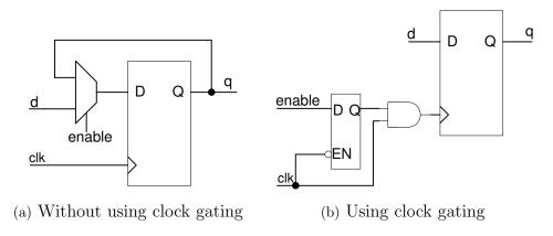
Figure 4.23 Implementation comparison between a flip-flop without clock gating and with clock gating.
