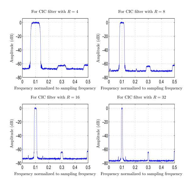
Figure 6.6 Output signal spectrum of the designed modulator with  $f_{out} \approx 0.1 \times f_{refclk}$ .
