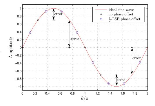
**Figure 4.4** Error comparison between no phase offset and  $\frac{1}{2}$ -LSB phase offset.
