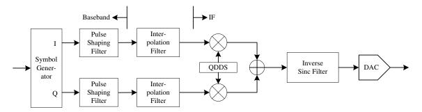
**Figure 2.1** Digital quadrature modulator.
