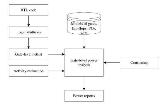
Figure 5.1 Power estimation in logic synthesizer.
