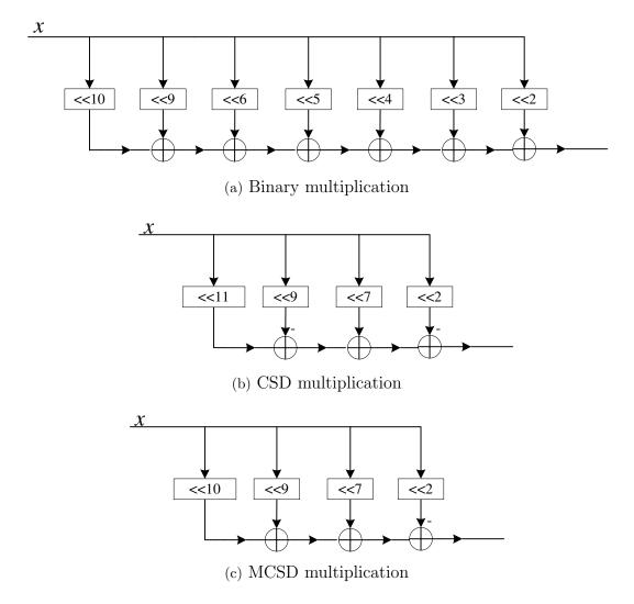
**Figure 4.22** Comparison of the three different ways to implement  $x \times h(4)$ .
