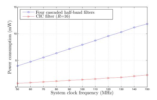
Figure 5.10 Power consumption comparison for two interpolation filters with the interpolation ratio of 16.
