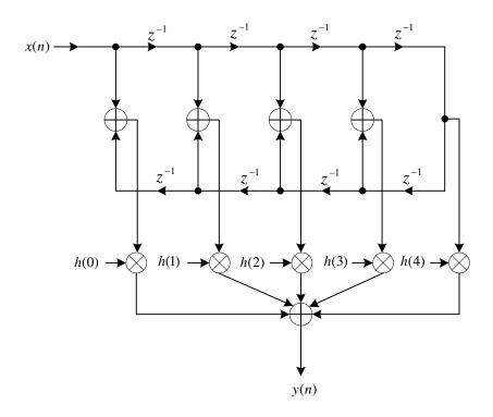
Figure 4.21 Signal flow graph of symmetrical FIR filter.
