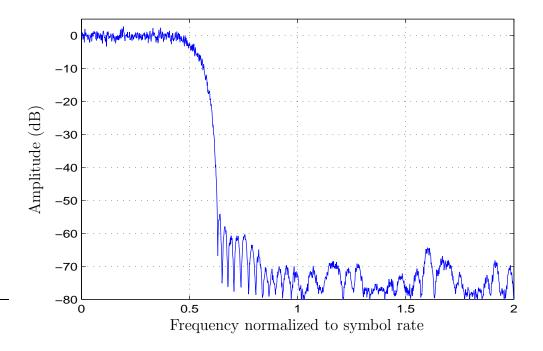
Figure 6.3 Signal spectrum after pulse shaping filter.
