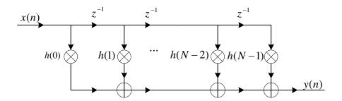
Figure 2.5 Signal flow graph of the direct form structure FIR filter.
