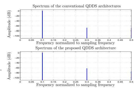
Figure 5.3 Spectrum of the QDDS output  $(f_{out} \approx 0.1 \times f_{refclk})$ .
