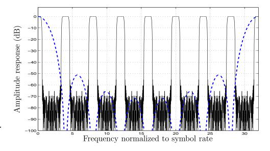
Figure 4.15 Spectral response of 1-to-8 CIC interpolator. Solid line shows the periodic spectrum of the zero packed time series and dashed line shows the frequency response of the CIC filter with rate change factor of 8.
