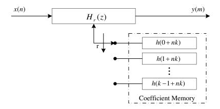
**Figure 4.9** An efficient implementation of 1-to-k upsampling polyphase filter.
