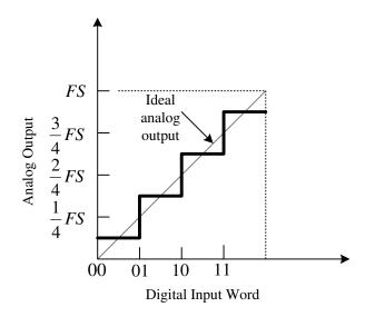
Figure 2.14 Ideal input output characteristics for a 2 bit DAC.
