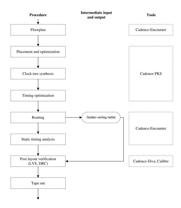
Figure 3.3 Block diagram of the back-end design flow.
