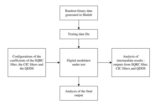
Figure 6.1 Testing model.
