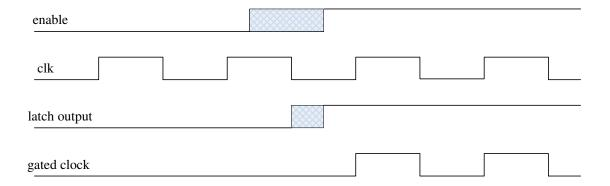
Figure 4.24 The mechanism of using latch to prevent the glitch on the gated clock net.
