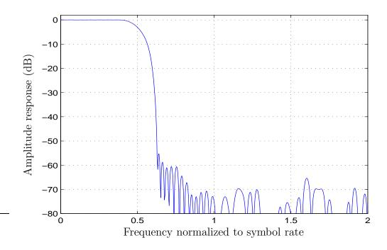
Figure 4.11 The frequency response of the SQRC filter whose impulse response is shown in Figure 4.10.
