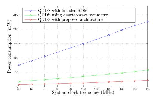
Figure 5.5 Power consumption comparison for 3 different QDDS architectures.
