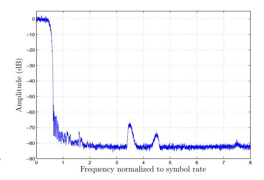
Figure 6.4 Signal spectrum after CIC filter (R = 4).
