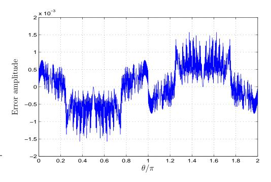
Figure 4.7 Errors for QLA sine phase to amplitude converter.
