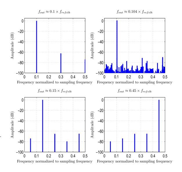
Figure 6.2 Spectrum of QDDS outputs.
