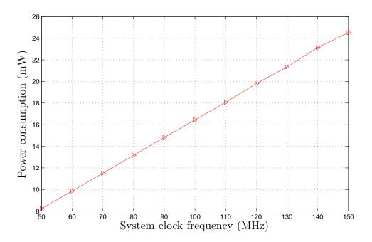
**Figure 6.8** Power consumption estimation of the designed modulator after logic synthesis.
