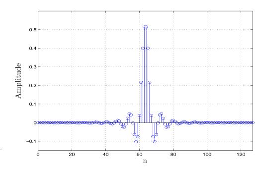
Figure 4.10 An example of the SQRC impulse response.
