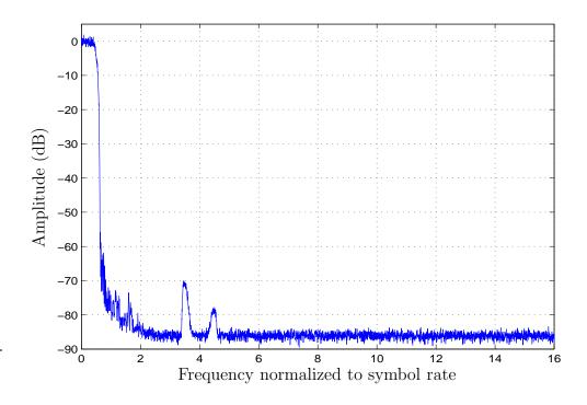
Figure 6.5 Signal spectrum after CIC filter (R=8).
