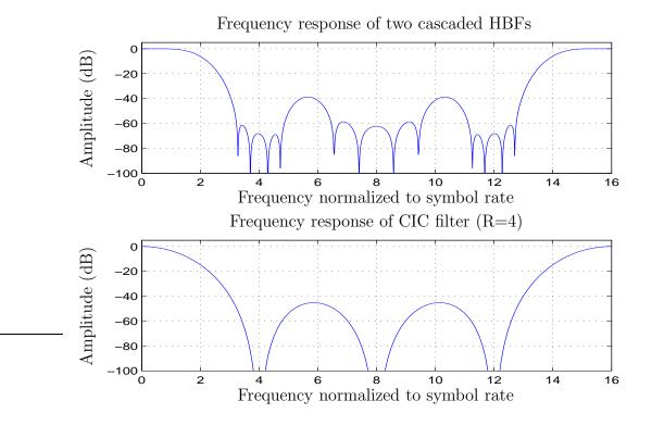
Figure 5.7 Comparison of HBF and CIC frequency response.
