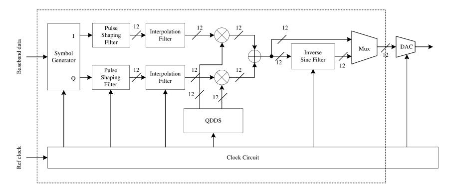
Figure 4.1 The detailed block diagram of the designed quadrature digital modulator.
