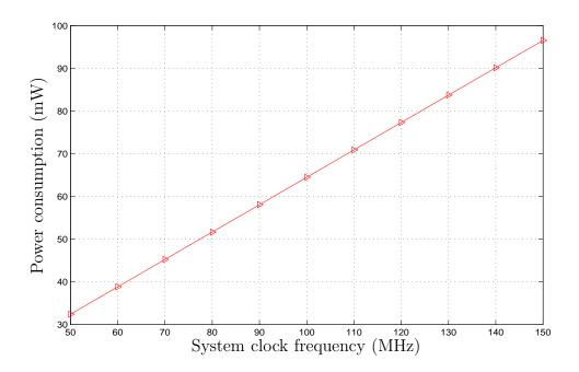
Figure 6.10 Power consumption estimation of the designed modulator after layout.
