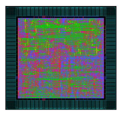
Figure 6.9 Layout of the designed modulator.
