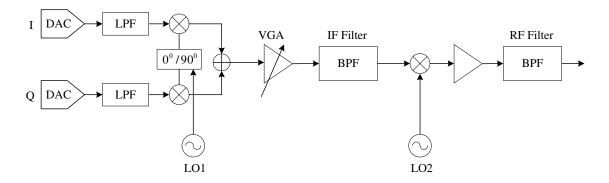
Figure 1.1 Analog transmitter.
