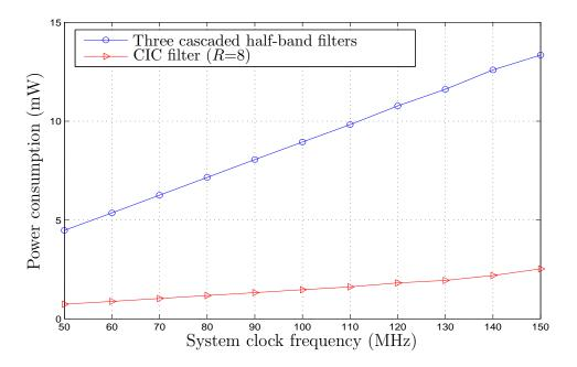
**Figure 5.9** Power consumption comparison for two interpolation filters with the interpolation ratio of 8.
