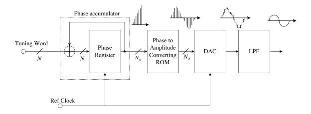
Figure 2.2 Block diagram of a basic DDS.
