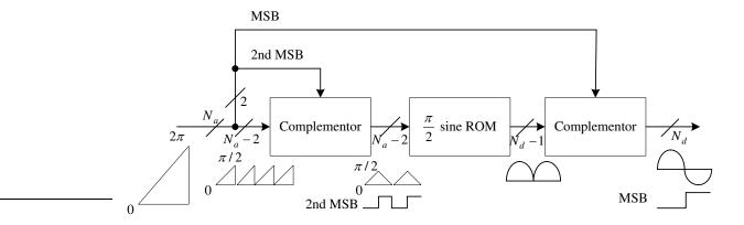
Figure 4.2 ROM design using quarter-wave symmetry.
