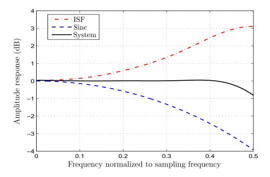
Figure 4.20 Frequency responses of the sinc distortion, ISF and the combined system.
