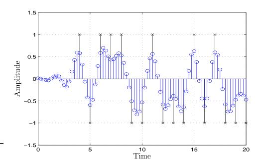
Figure 2.7 Output sequence of a SQRC filter. "x" shows the input binary data and "o" shows the output sequence.
