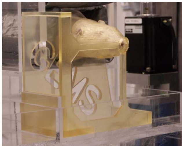
Figure 3.18 Rat head restraint fabricated by a rapid prototyper
