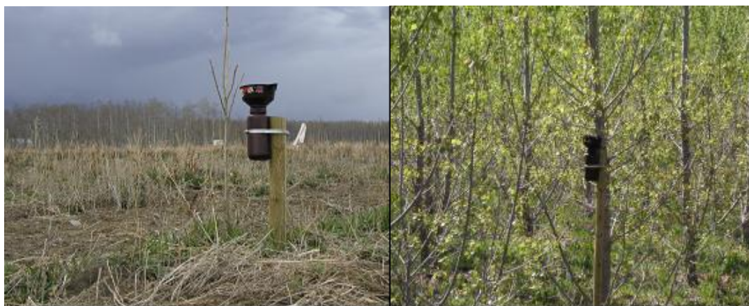
Figure D.1. Throughfall collector mounted on 1 m high fencepost under a four-year-old tree at the Pasture site in May, 2004 (left) and underneath a seven-year-old tree at the Alfalfa site in June, 2004 (right).
