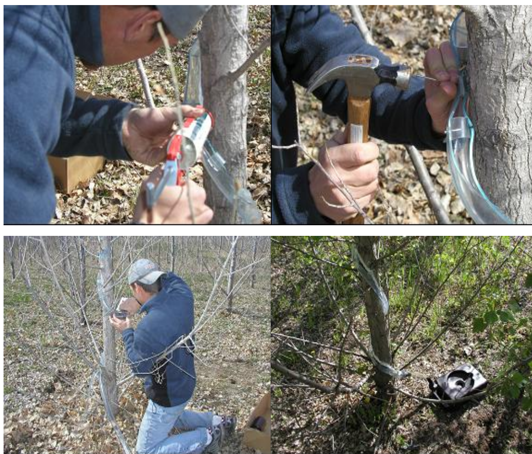
Figure D.2. Stemflow collection installation on the bole of a seven-year-old tree in the Alfalfa plantation. The tubing was nailed and stapled to the tree (top left and right) and then caulked so no gap existed between the tree and the tubing (bottom left) and then attached to a 10 L plastic container to collect the stemflow solution (bottom right).
